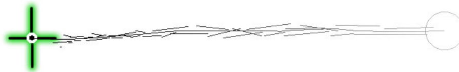
Figure 30: Modified Touch + Trace visualization. Note the faded circle on the right at the point of contact. Over time, the circle fades and expands, simulating a ripple.
