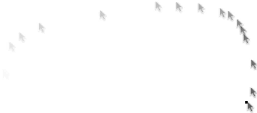
Figure 70: Temporal traces using a mouse pointer as a graphical icon. The current location of the gesture is the embodiment with the small square at the end of the pointer (bottom, right).
