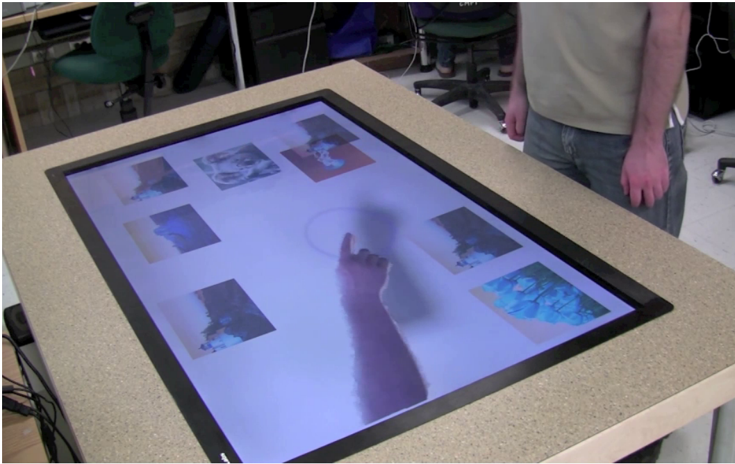
Figure 38: Simulated use of KinectArms in a photo-sharing application, showing shadow and height indicator (circle).
