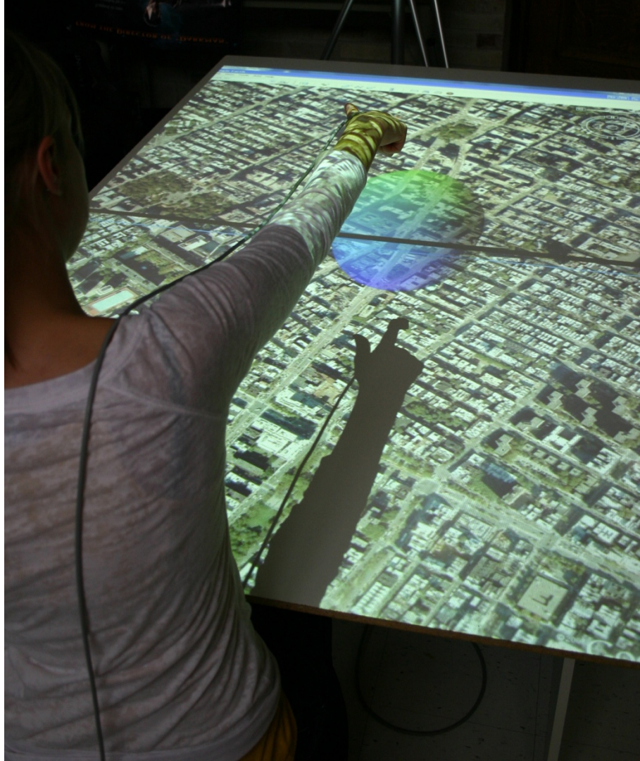
Figure 24: The top-down projected table used for study 1, study 2, and by the local participant in study 3. In this image, the user is seated at the foot of the table, as were participants in all of the studies. The black line in the middle of the table is where the stitch between the two projector images.
