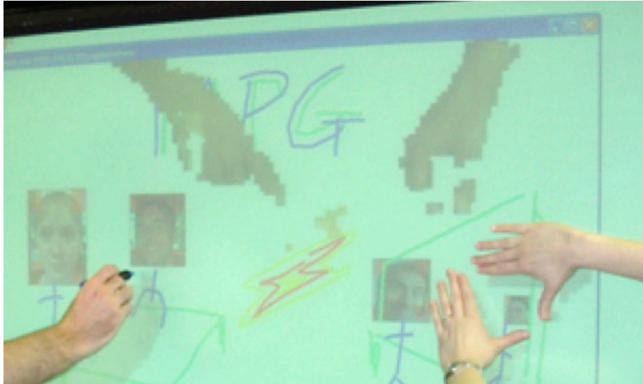
Figure 56: VideoArms in use. The embodiments are blocky and have interrupted boundaries, possibly making it difficult to interpret a gesture.
