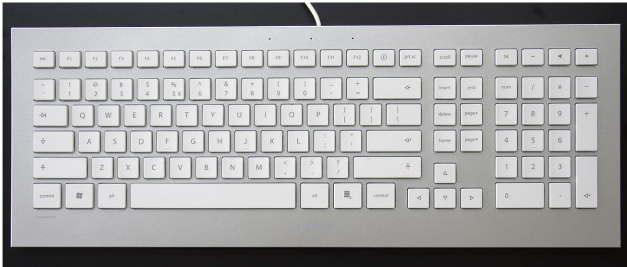
Figure 2.2.4: A standard wired chiclet style keyboard [54].
