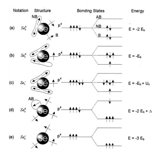
**Figure B.1** Structure and energy of simple bonding configuration for selenium atoms. Straight lines represent bonding orbitals, lobes represents lone-pair (nonbonding) orbitals, and circles represent antibonding orbitals. The energy of lone-pair is taken as the zero energy (Ref. 50).
