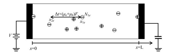
**Figure 4.7** Schematic illustration showing positions  $x_1$  and  $x_2$  for bimolecular recombination within time interval  $\Delta t$ .
