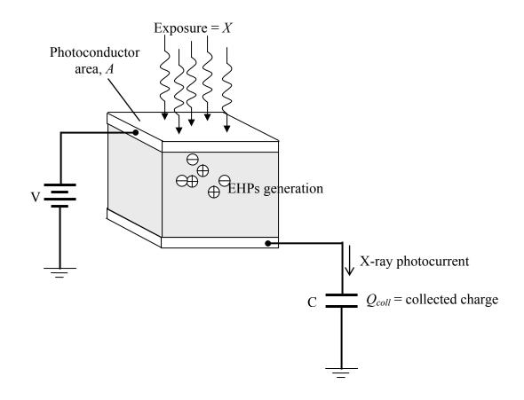
**Figure 3.1** Schematic illustration of the photoconductor sandwiched between two parallel plate electrodes.
