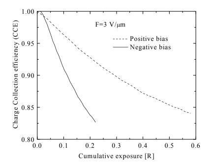
Figure 5.29 The charge collection efficiency versus cumulative exposure for both positive and negative biasing conditions. The applied electric field is 3  $V/\mu m$ .
