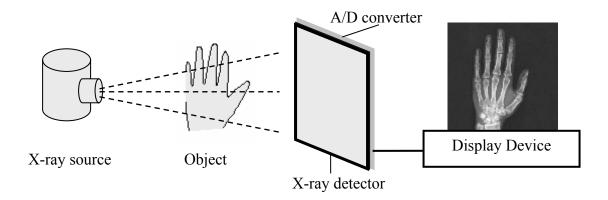
**Figure 1.3** Schematic illustration of a digital radiography system.
