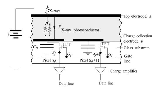
**Figure 1.10** Cross sectional structure of a flat panel active matrix direct conversion x-ray image detector (two pixels).
