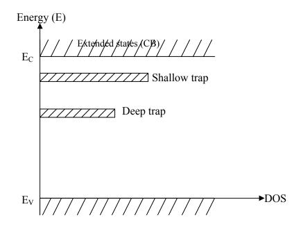
**Figure 3.8** Schematic illustration of shallow and deep traps for electrons in amorphous semiconductors.
