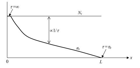
Figure 4.10 Schematic illustration of trap filling effect.
