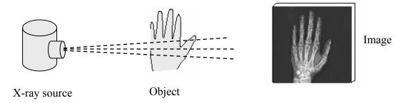
**Figure 1.1** A typical radiographic x-ray imaging technique.
