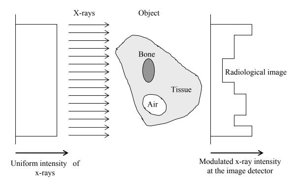
**Figure 1.2** Schematic diagram of differential attenuation of x-rays in human body.
