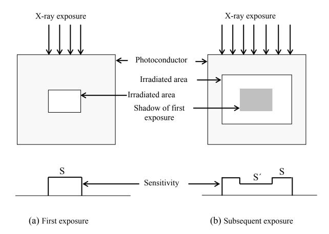
**Figure 1.11** Schematic illustration of ghosting in x-ray photoconductors.
