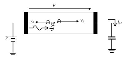
**Figure 3.7** Schematic illustrations of carriers drift and current in a positively biased x-ray photoconductor.
