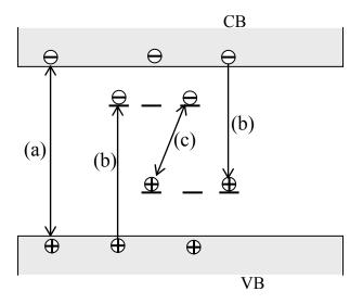
**Figure 1.12** Schematic diagram of possible electron hole recombination process in a-Se.
