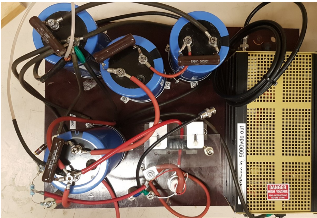
Figure 4.13: Pulsed Power Supply (Internals)
