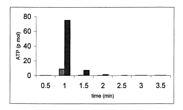
**Fig.3.5** ATP dilution in the chamber of 0.15 ml volume and outflow provided by a vacuum pump. 4.6 nl and 46 nl of 1 mM ATP were injected into the chamber. Amounts of ATP in 30-s samples collected before and after injection shown by gray (4.6 nl injected) and dark (46 nl injected) bars. ATP was detected in 2-3 30-s samples after injection. ATP was injected in the beginning of the collection of the second sample. The perfusate flow rate was 1 ml/min.
