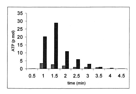
**Fig.3.4** ATP dilution in the chamber of 0.3 ml volume and outflow provided by gravity force. 4.6 nl and 46 nl of 1 mM ATP were injected into the chamber. Amounts of ATP in 30-s samples collected before and after injection shown by gray (4.6 nl injected) and dark (46 nl injected) bars. ATP was detected in 6-7 30-s samples after injection. ATP was injected in the beginning of the collection of the second sample. The perfusate flow rate was 1 ml/min.
