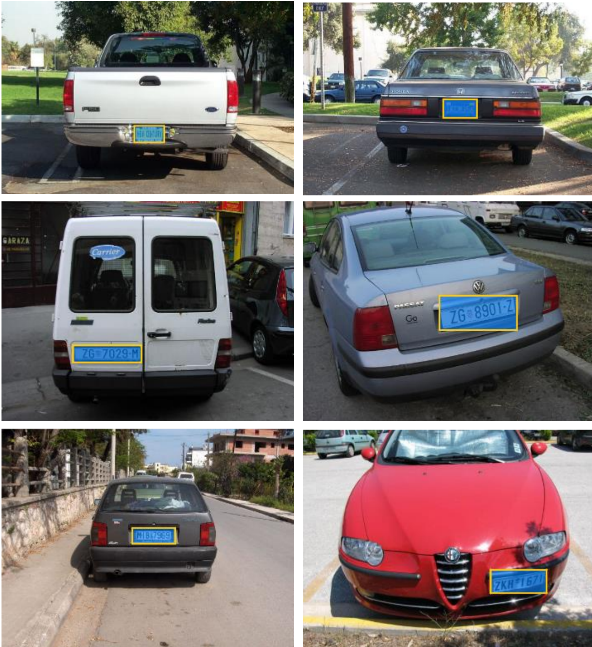
Figure 4.3: Images of plate regions on vehicles labelled using labelImg [92] (with emphasis added by manually drawing yellow boxes around the labelled plate region). From each of these, a respective XML file will be generated for record creation and training/testing. The first row contains images from the Caltech dataset [96], the second row from the University of Zagreb dataset [100], and the third from the NTUA Medialab dataset [102].
