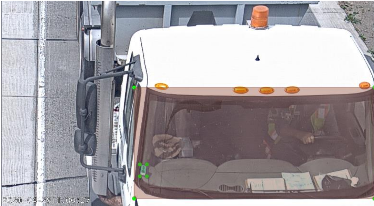
Figure 5.3: Windshield and CVSA decal labelled using the LabelImg program.
