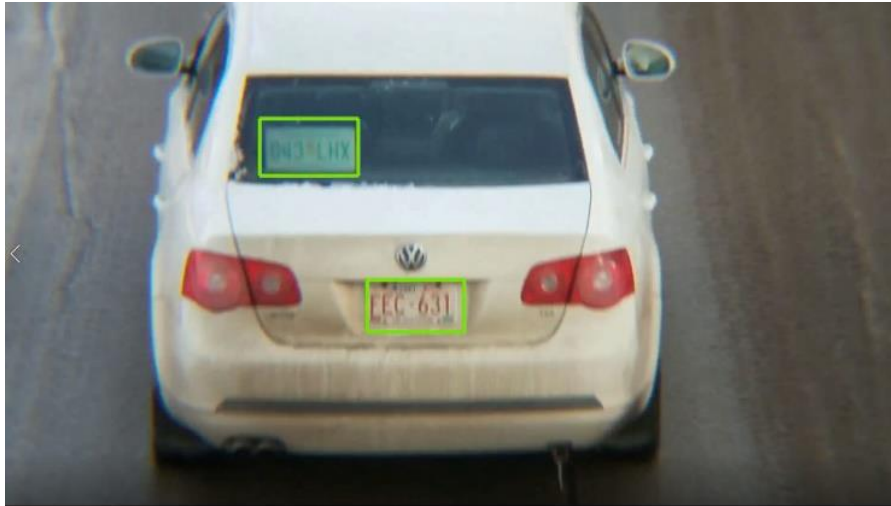
Figure 4.8: Real-time can detect one or multiple license plates at the same time.
