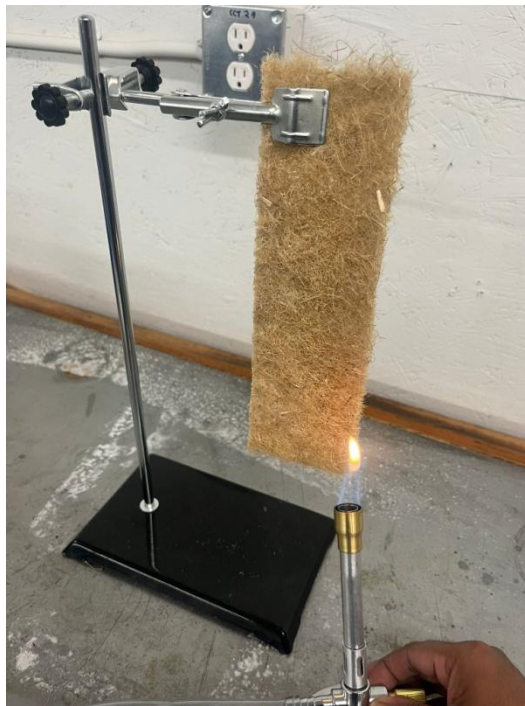
Figure 4.13 Experimental setup for flame resistance test of the nonwoven hemp fiber fabric
