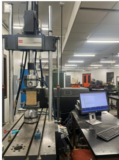
Figure 4.14 Experimental setup for Tensile strength test of the nonwoven hemp fiber fabric
