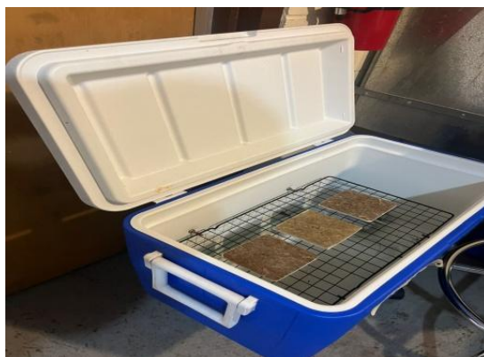
Figure 4.23 The sample conditioner for cone calorimeter test
