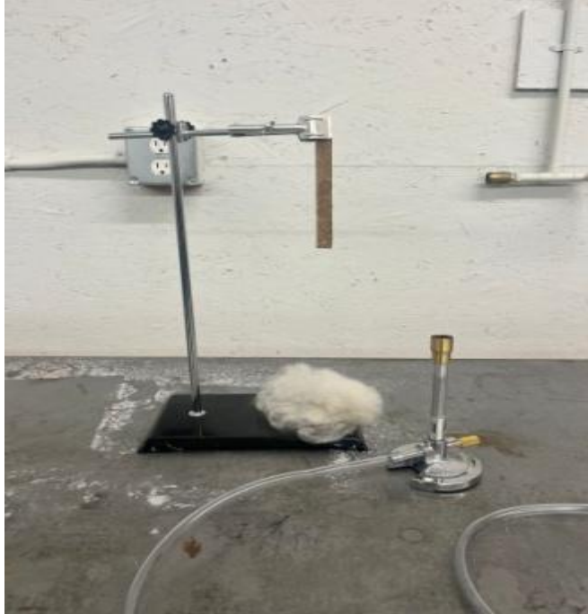
Figure 4.22 The experimental setup of UL94 vertical burn test
