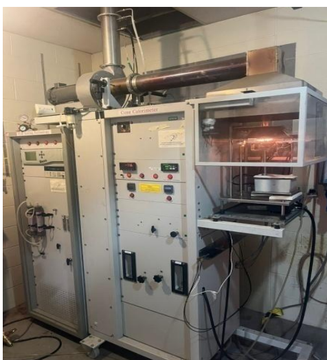
Figure 4.24 The cone calorimeter
