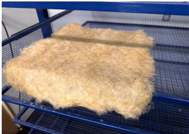
Figure 4.9 Natural drying of hemp fiber fabric after APP treatment
