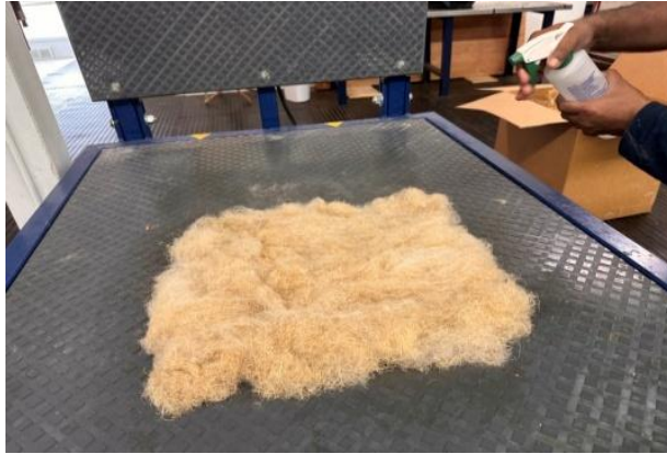
Figure 4.8 Fiber batting on the pressing machine
