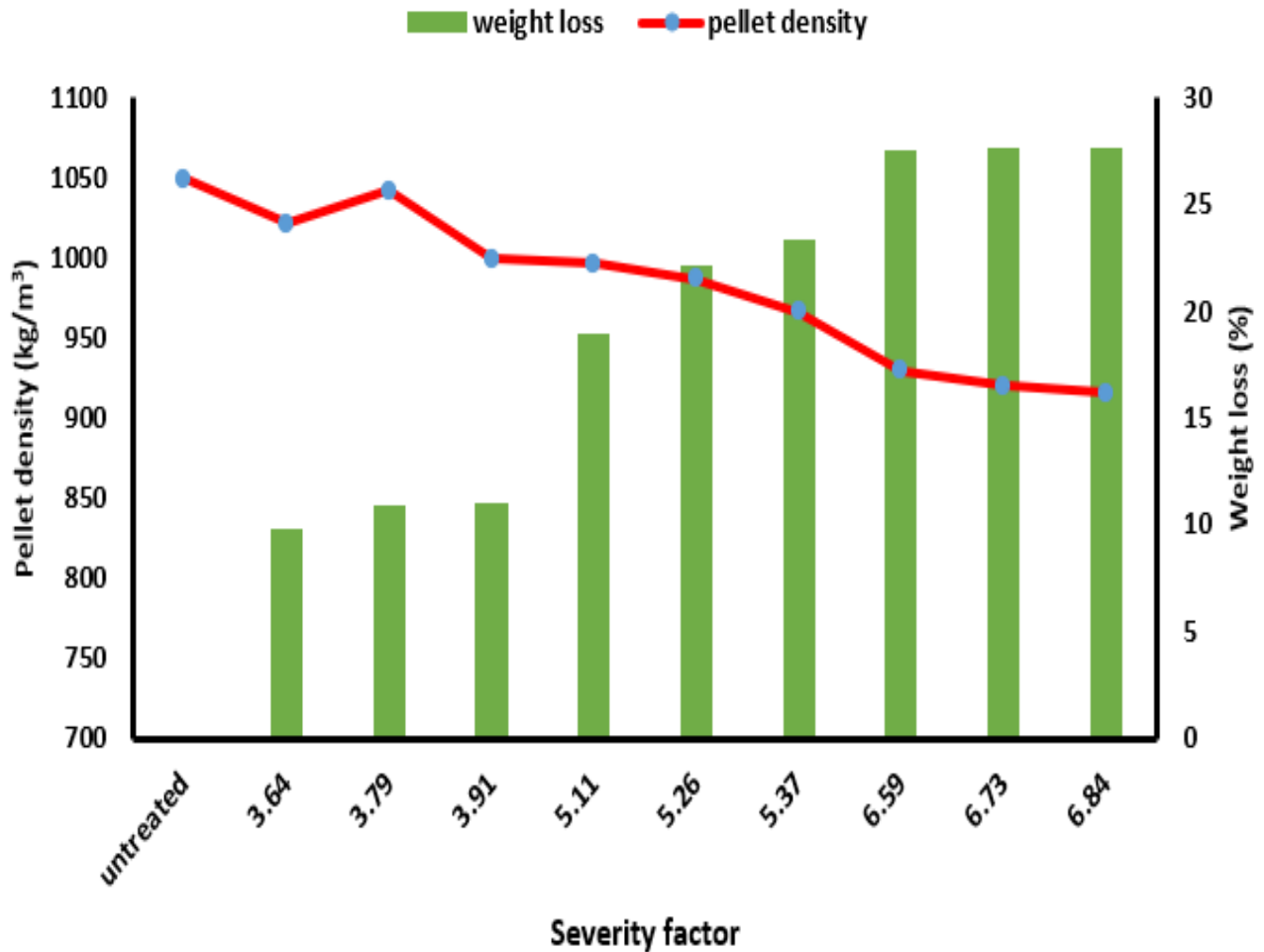
Figure 4.7. Pellet unit density and weight loss of raw WSS and WSS biochar for different severity factors.
