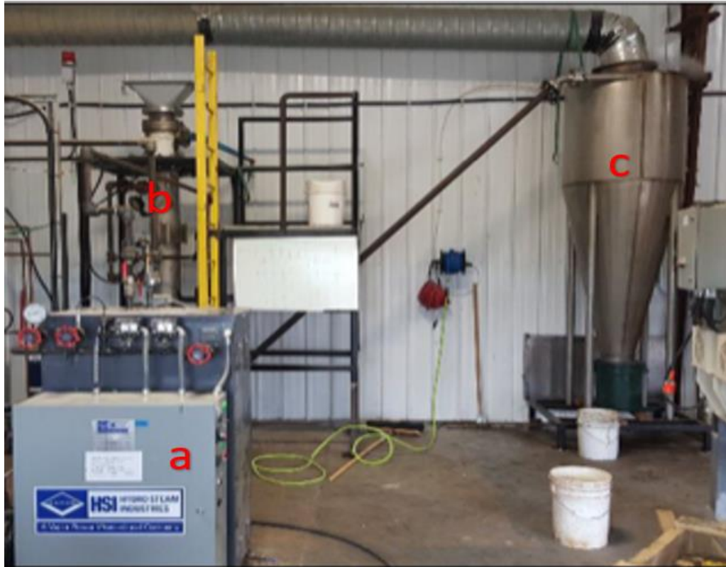
Figure S3.1. Photographs of the steam explosion system used in the experiments. (a) steam generator; (b) pressure vessel (chamber); (c) cyclone.
