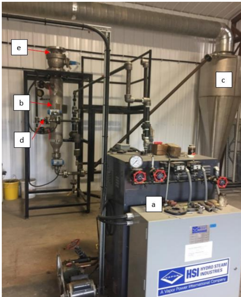
Figure 2.4. Steam explosion system at the Canadian Feed Research Centre, University of Saskatchewan.
