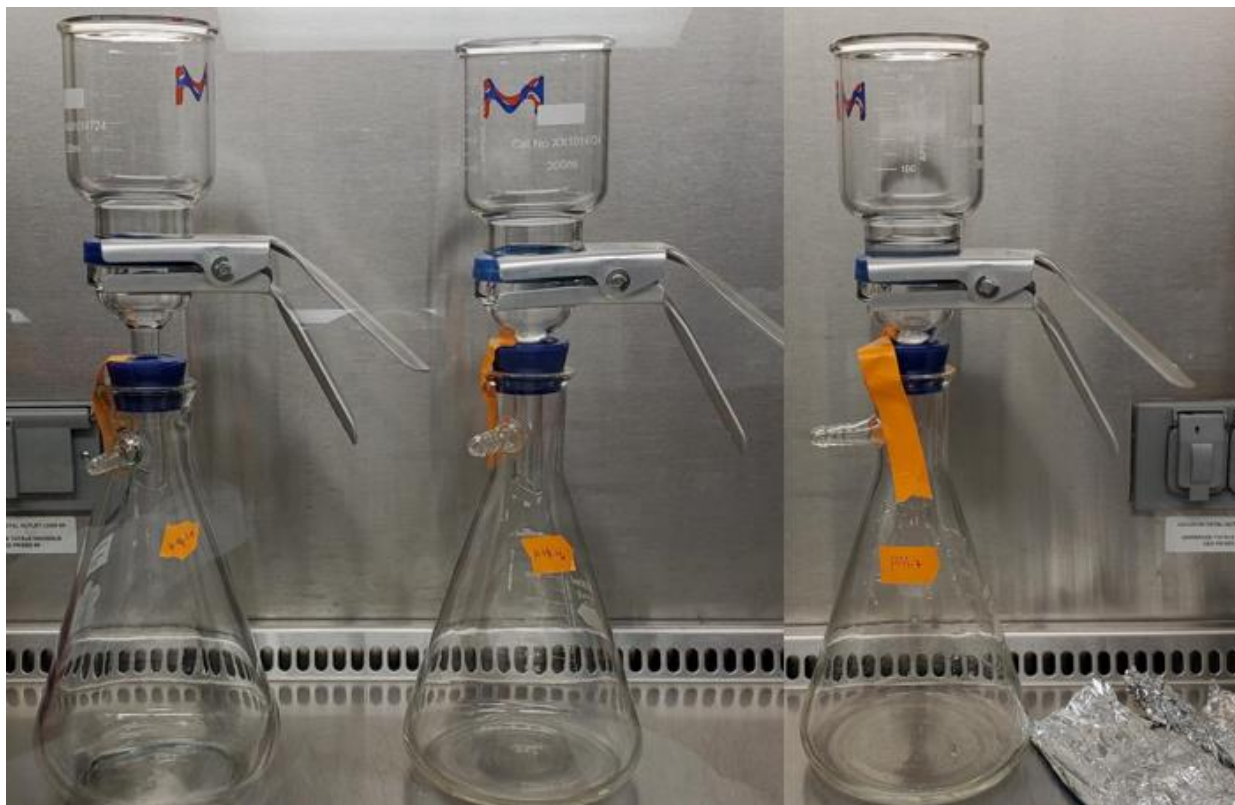
Figure 5.2. Cell-filtration using Millipore Vacuum Manifold (Millipore Inc., Bedford, MA), Microfil Filtration Funnels and S-Pak 0.45-mm Type HA membranes (Millipore Inc.). An accu-jet ® pro pipette controller was used to remove air through the nozzles of each filter flask and aid the filtration.
