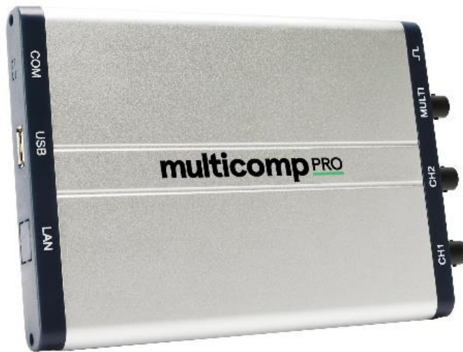
Figure 2-5: Data Acquisition Unit, Model-Multicomp (MP720646 US)
