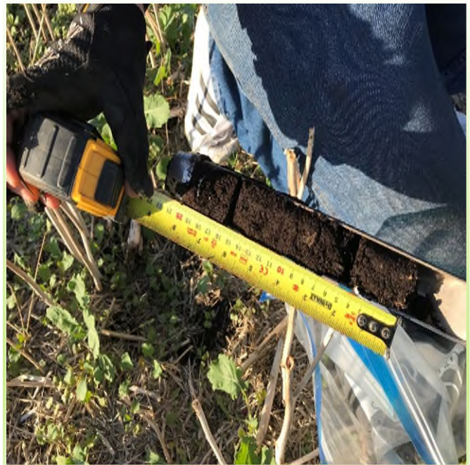
Soil sampling in the field, as the first step for laboratory tests.
