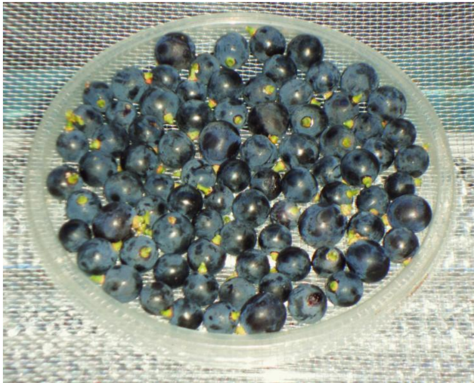
Figure 3.4 UV-C irradiation of grape berries with pedicels attached. Berries are resting directly on an aluminum screen with lamps placed above and below. Plastic hoop is in place to prevent samples from rolling.
