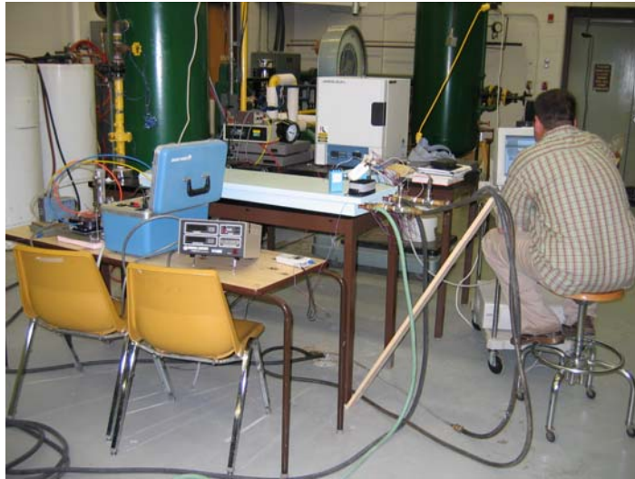
Figure B.4 Calibration of the relative humidity sensors using the Hydro-MZ dew point monitor.
