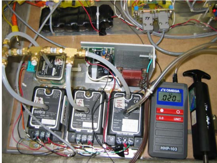
Figure B.5 The pressure transducers and calibration of the sensors using the OMEGA pressure meter and pump.
