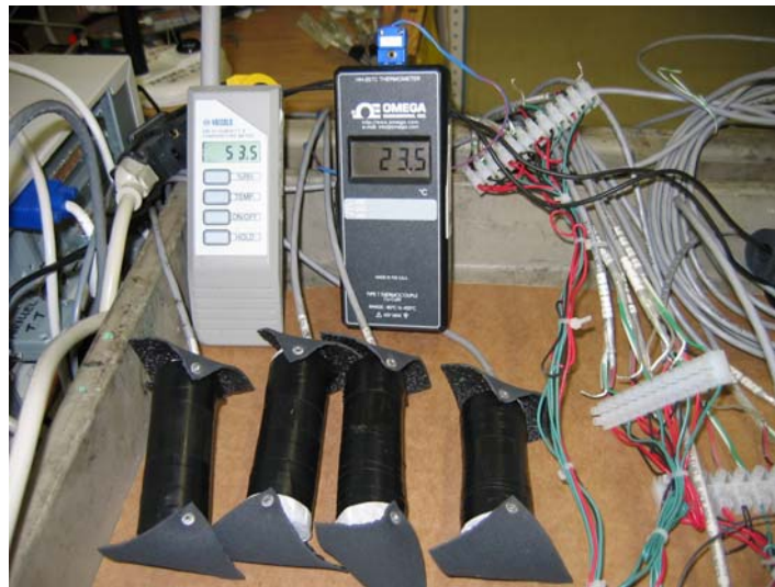
Figure B.3 The relative humidity sensors covered with PVC covers.
