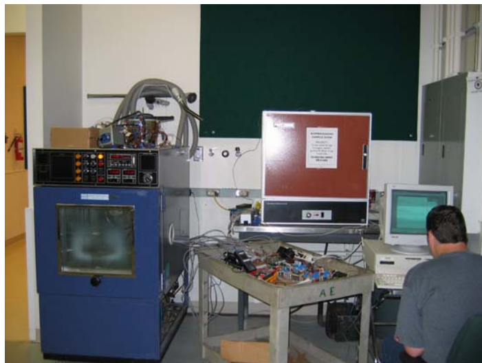
Figure B.2 Calibration of the temperature sensors using the angelantoni climatic system.
