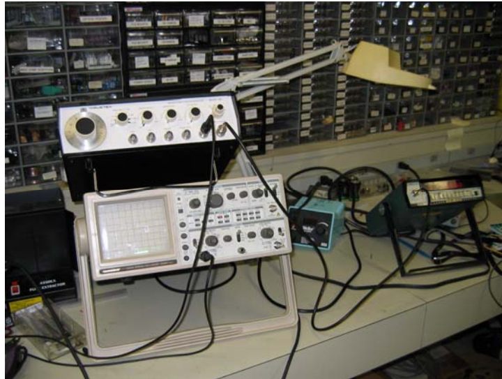
Figure B.6 Calibration of the Hall fan sensors using the 50-MHz pulse generator and 1.3-GHz frequency counter.
