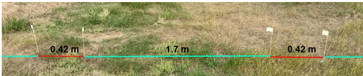
Figure 4.3: Annotated close-up of the plot markings: the length of the plot edge (1.7 metres) is depicted by the green lines, and the distance between two plots (0.42 metres) is depicted by the red lines.
