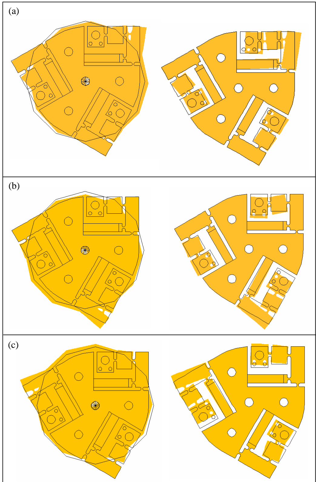
Figure 3.17 The deformation of the RRR mechanism by activating the single PZT actuator (a: PZT 1; b: PZT 2; c: PZT 3).
