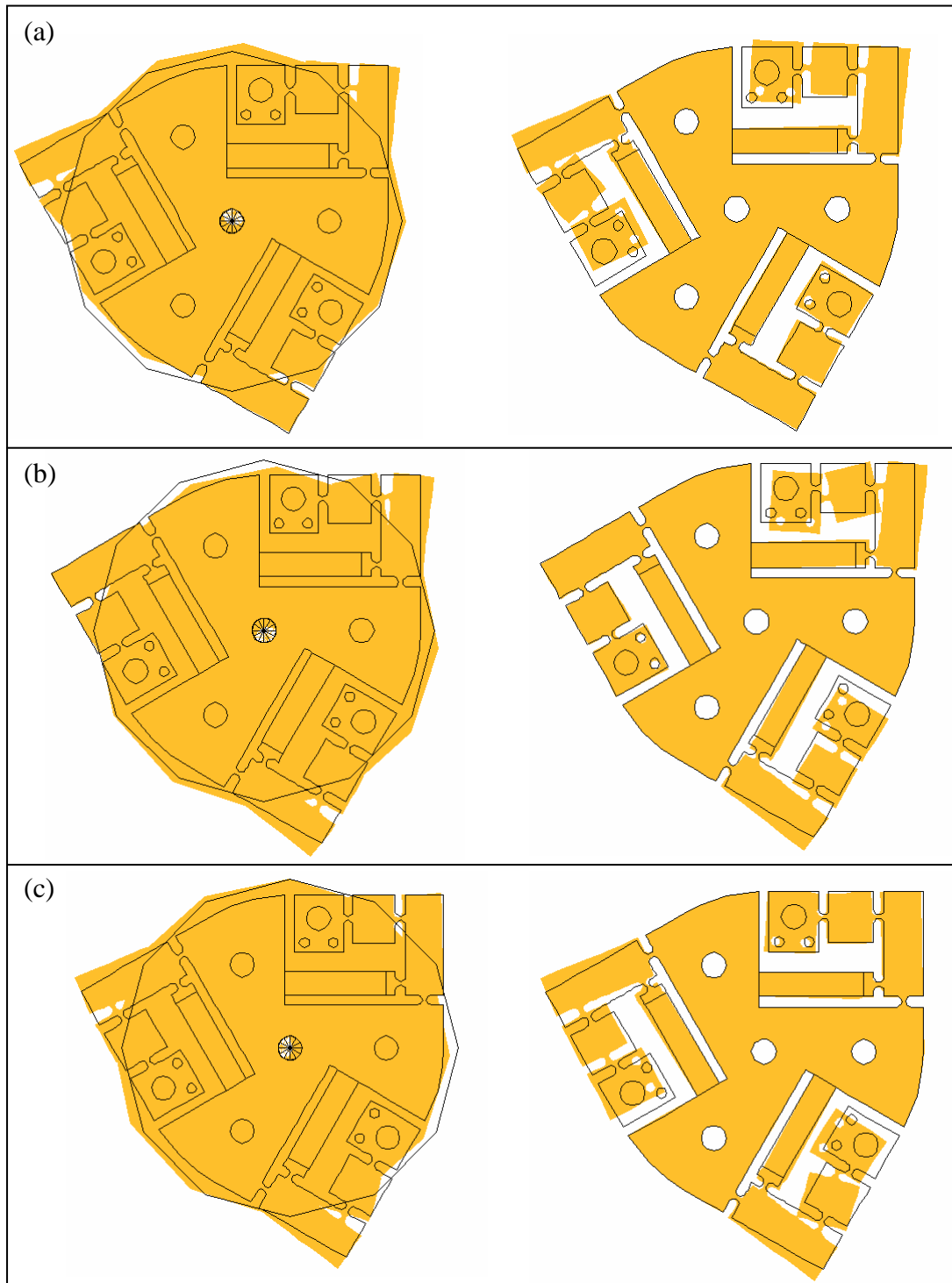
Figure 3.18 The deformation of the RRR mechanism by activating two PZT actuators (a: PZT 1 and 3; b: PZT 1 and 2; c: PZT 2 and 3).
