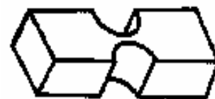
Revolute joint type in compliant body (Flexure hinges)
