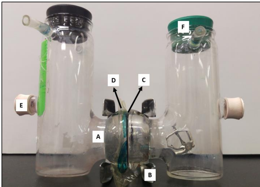
Figure 3.3 Microbial Fuel Cell components. (A) Flanged glass extension (B) Metallic clamp (C) Rubber O Ring (D) Nafion high exchange capacity proton exchange membrane (E) Sampling port (F) Rubber stopper.
