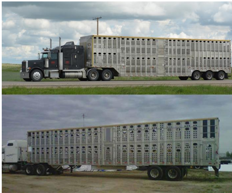
Figure 2.1. Pot belly (top) and straight deck (bottom) livestock trailers commonly found in Canada. Figures obtained from www.robergeinc.com , www.thepigsite.com .
