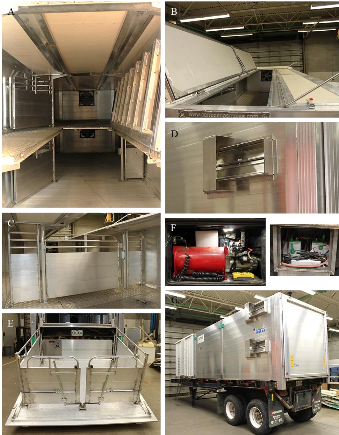
Figure 3.3. Photos of the animal compartment showing (A) its lower and upper decks, (B) hinged roof, (C) gate that partitions one deck into two pens, (D) air exhaust damper, (E) hydraulic lift gate, (F) hydraulic lift controller and (G) compartment exterior.
