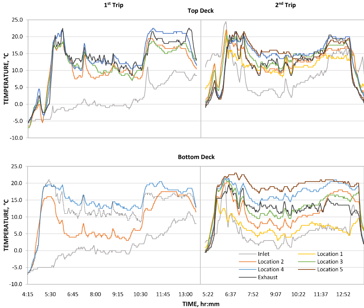
Figure 4.3. Variation in inlet, exhaust and internal trailer temperature measured at different locations approximately 1 m ( \approx 40 in) above the floor along the center of the trailer top and bottom decks during the two monitoring trips. The time series represent temperature levels from start of loading in the farm to end of unloading in the plant.
