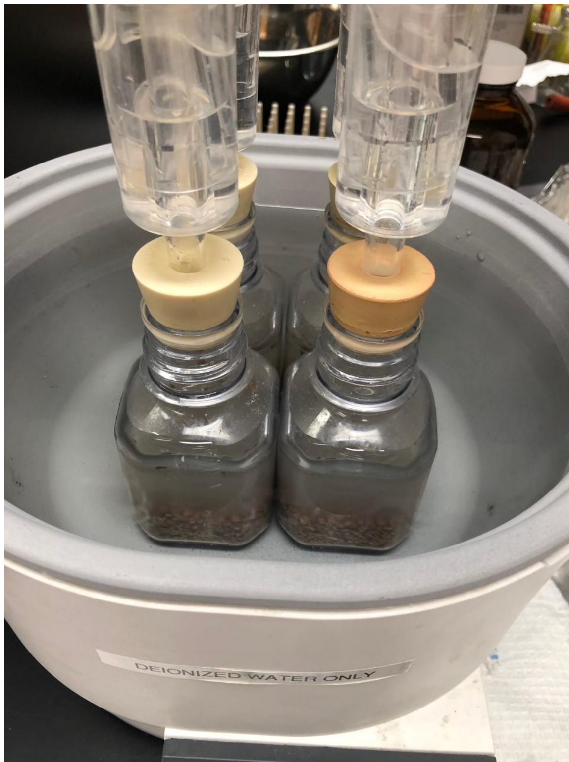
Figure S4. Bench-scale fermentation at 30 °C using a Büchi water bath B-490 (Flawil, Switzerland) for 72 h.
