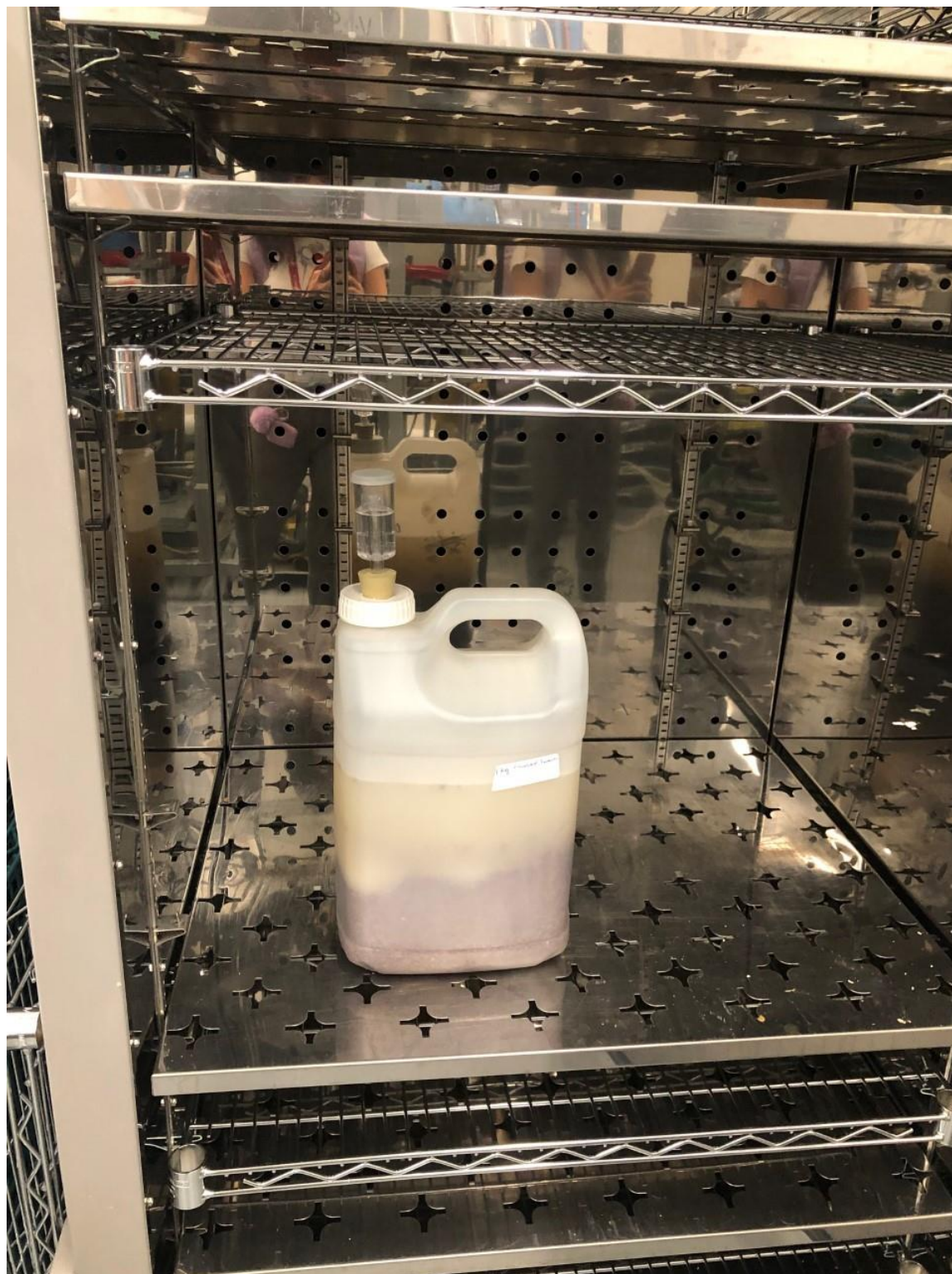
Figure S6. 1 kg flaxseed fermentation flaxseed fermentation in a VWR 1390FM mechanical oven incubator (Radnor, PA, USA) at 30 °C for 72 h.
