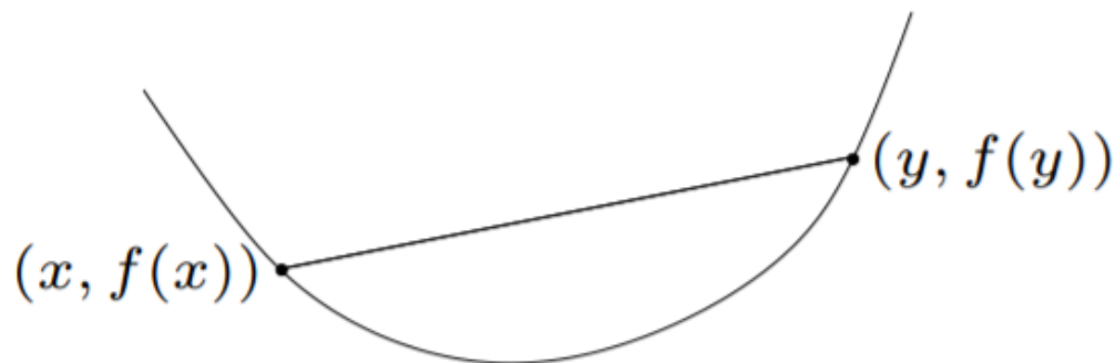
Figure 2.5: Graph of an example for convex function The chord from (x, f(x)) to (y, f(y)) , lies above the graph of f .
