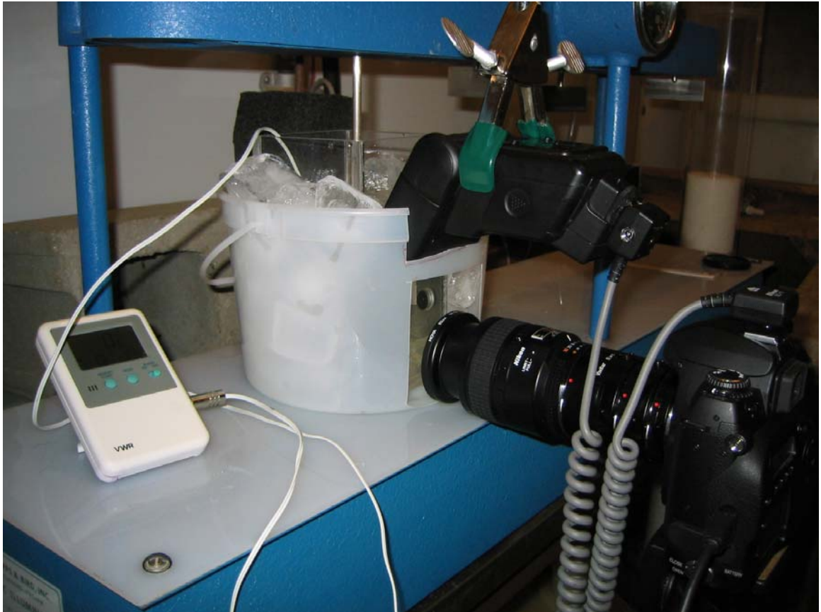
Figure 3.6. Experimental apparatus for the experiment at a water temperature of 0 °C in ECC
