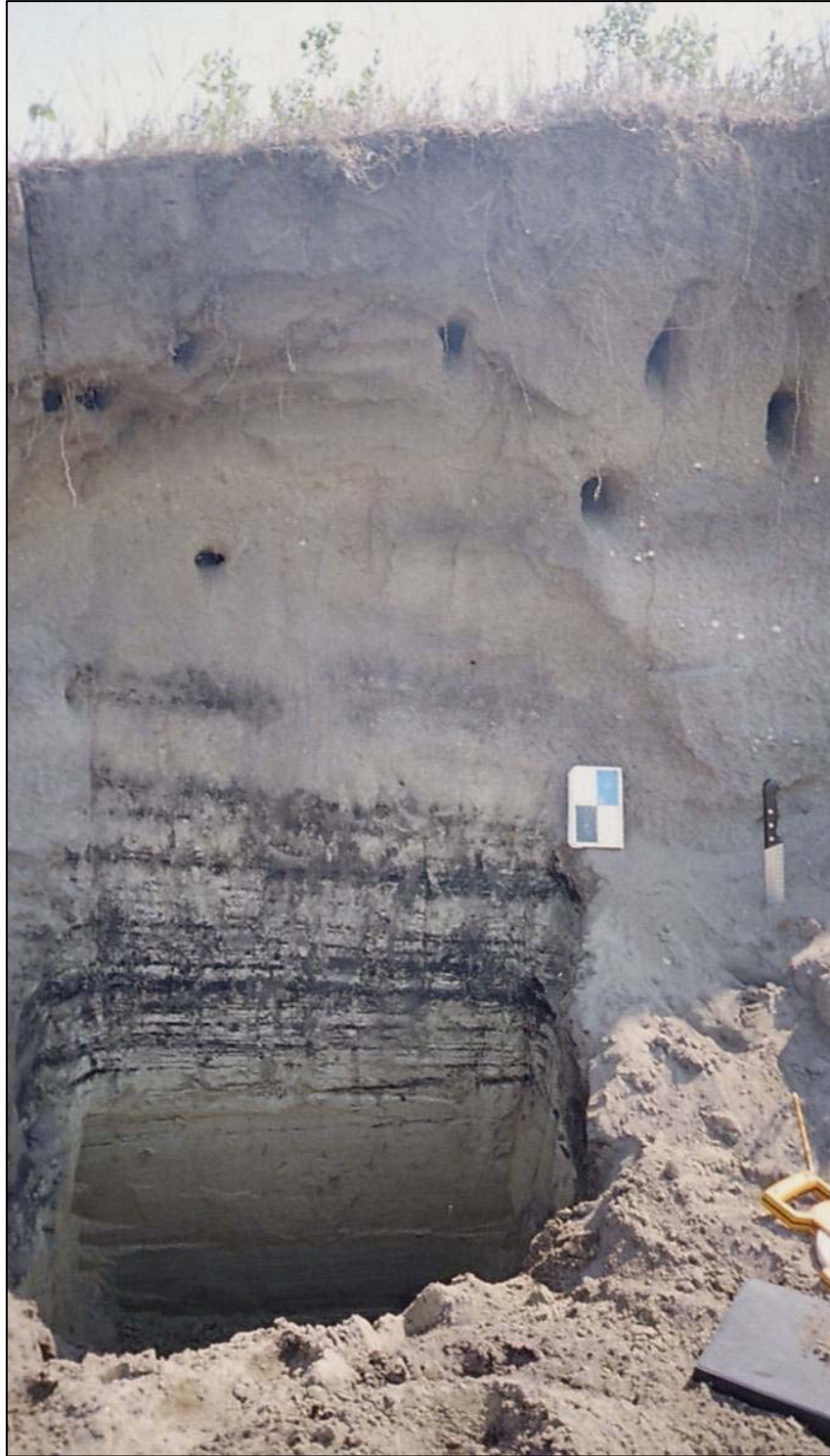
Fig. 5.2. Field photograph of the aeolian sand dunes type vertical profile. Note: field notebook in the photograph has the dimensions of 17.7 cm X 11.0 cm.
