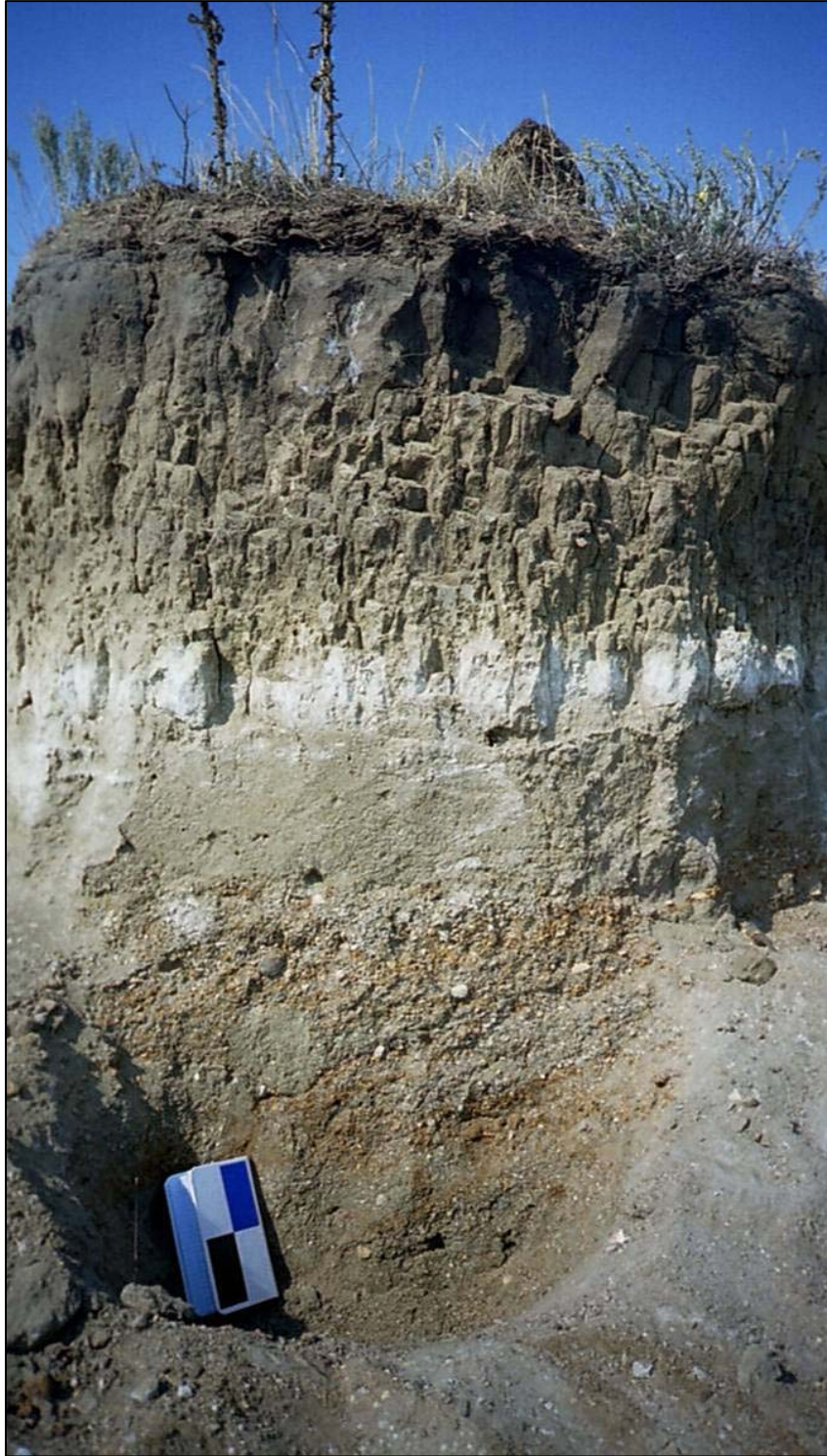
Fig. 5.6. Field photograph of the outwash plain type vertical profile. Note: field notebook in the photograph has the dimensions of 17.7 cm X 11.0 cm.
