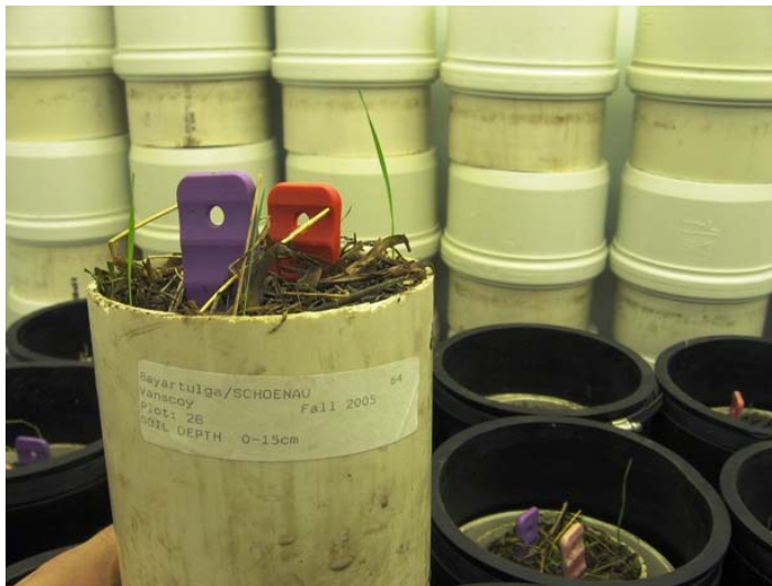
Figure 4. 1. Intact core with PRS™ probe inserted and ready to be placed into chamber.
