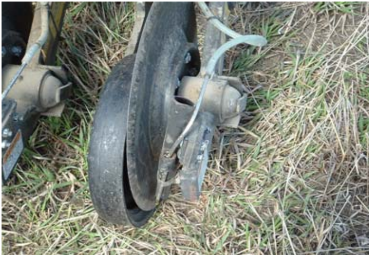
Figure 2 3. Coultter disk for fertilizer application.
