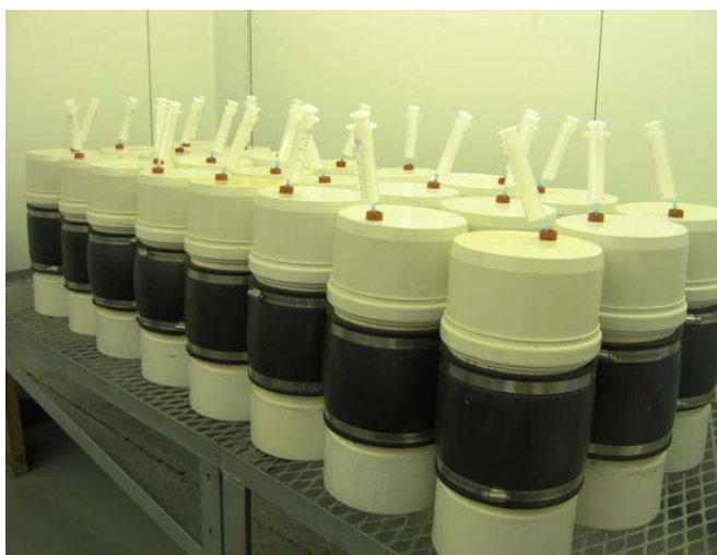
Figure 4. 2. Sealed chambers containing intact soil cores with syringe inserted ready for gas sampling
