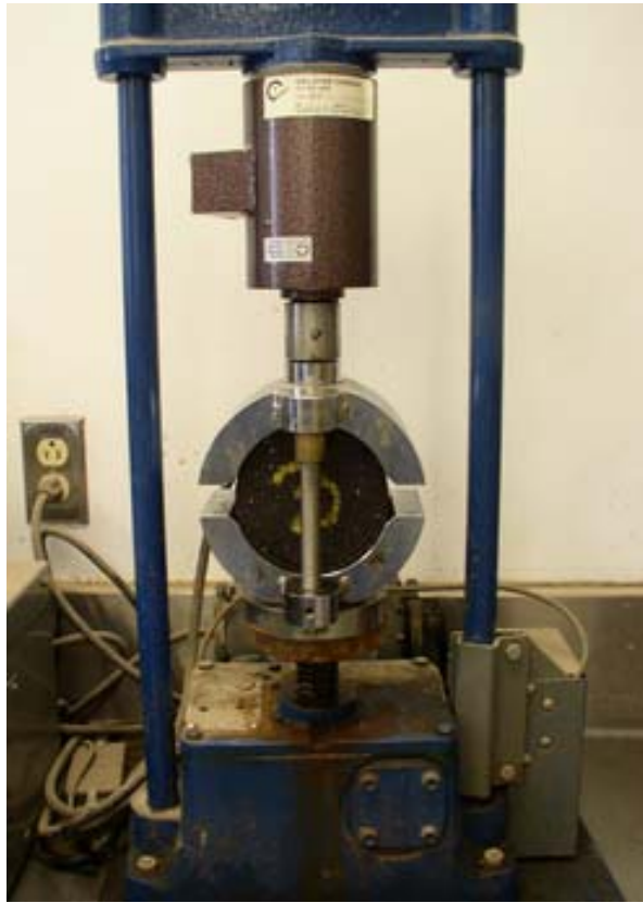
Figure 2.13 Marshall Stabilometer at the SDHT Laboratory
