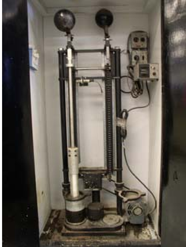
Figure 2.12 Marshall Compaction Apparatus at SDHT Laboratory
