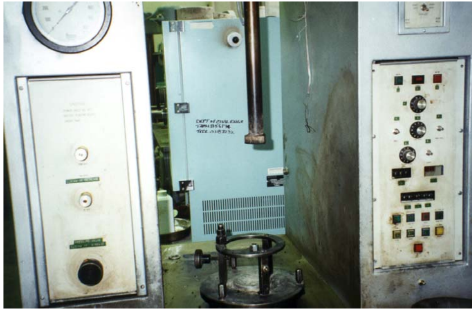
Figure 2.15 Hveem Kneading Compactor Foot and Rotating Base
