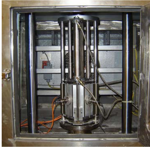
Figure 4.1 University of Saskatchewan Triaxial Frequency Sweep Equipment
