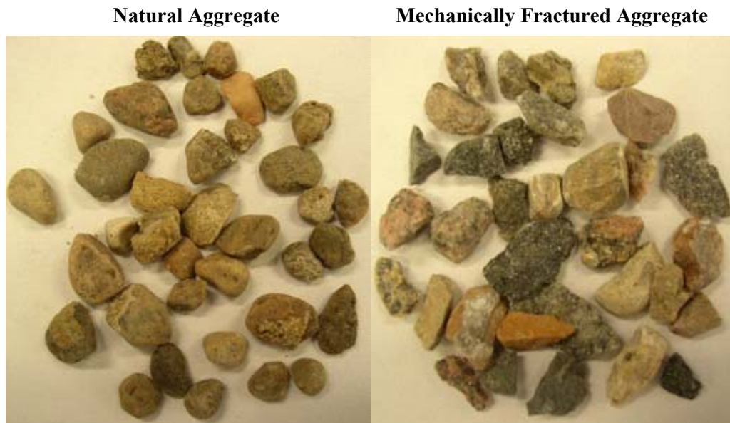
Figure 2.9 Effect of Mechanical Crushing on Aggregate Shape
