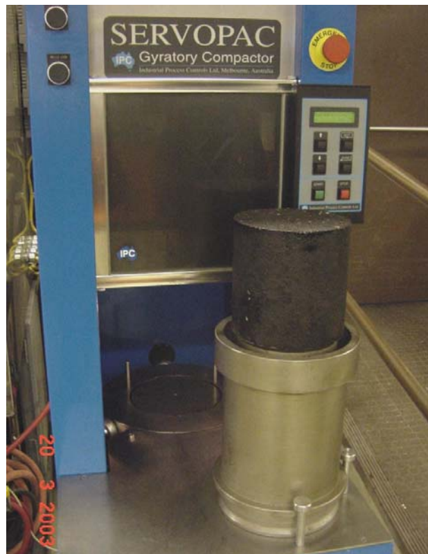
Figure 2.17 SHRP Gyratory Compactor with Compacted Sample
