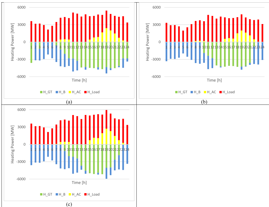
Fig. 5. Optimal heating power flow under scenario 2: (a) RA-IGDT method, (b) RS-IGDT method, (c) robust method.
