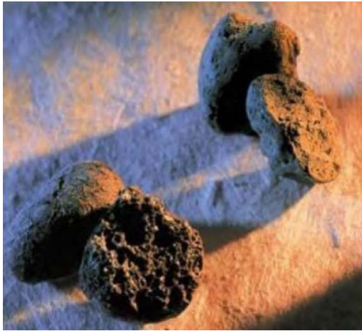
Figure 5.11 Bio-filter media in Yellow Quill treatment system (Neapetung, 2006).
