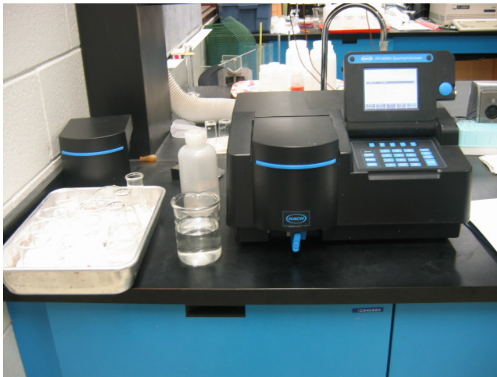
Figure 3.6 Hach DR/4000U UV/VIS spectrophotometer.
