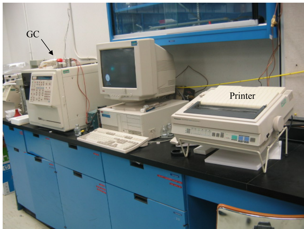
Figure 3.7 Varian star 3400CX Gas chromatographer with hp 7675A purge trap sampler.
