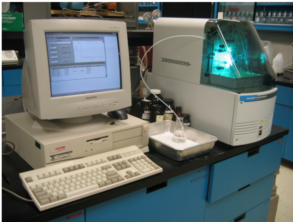
Figure 3.5 Phoenix 8000 UV-persulfate TOC analyzer.
