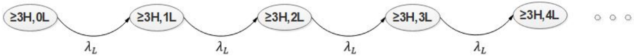
Figure 4.8: Markov chain of low-priority customers in the presence of at least three high-priority customers
