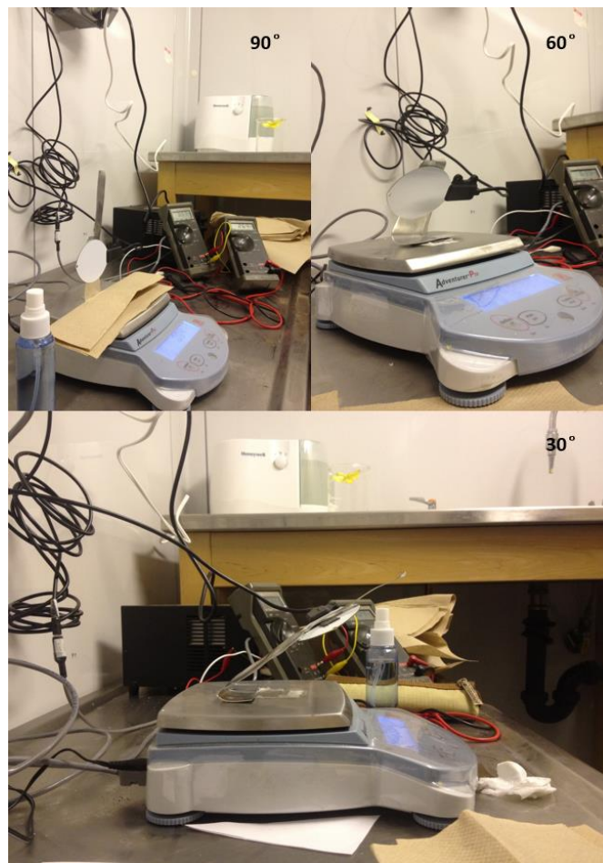
Figure 4.3. Test of the leaf wetness sensor at different angles.
