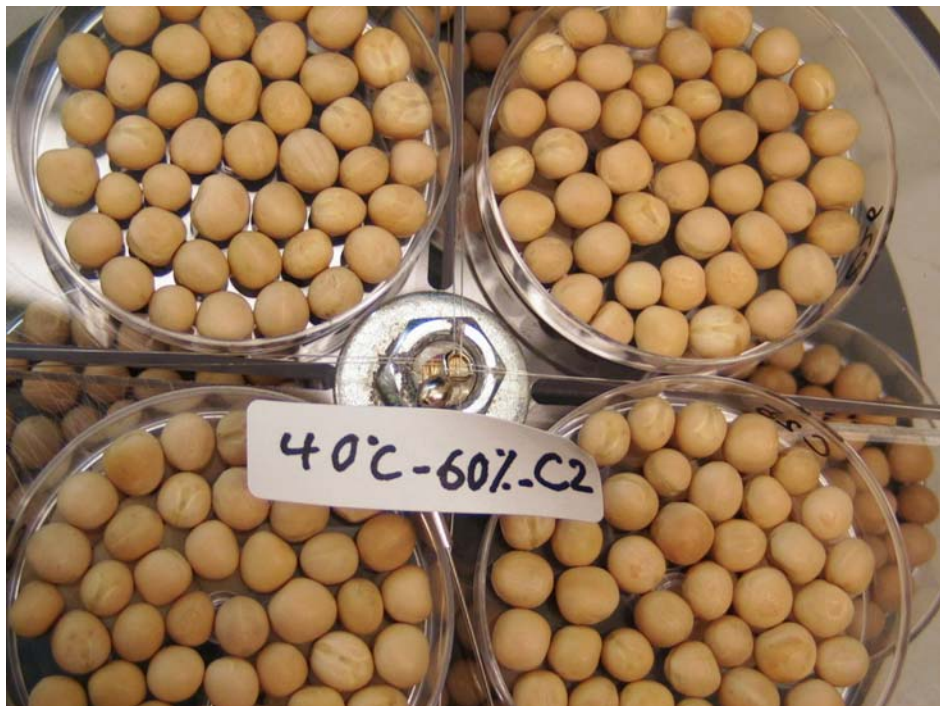
Figure E.9 Appearance of feed and clean peas after 174 days of storage at 40°C and 60% RH.
