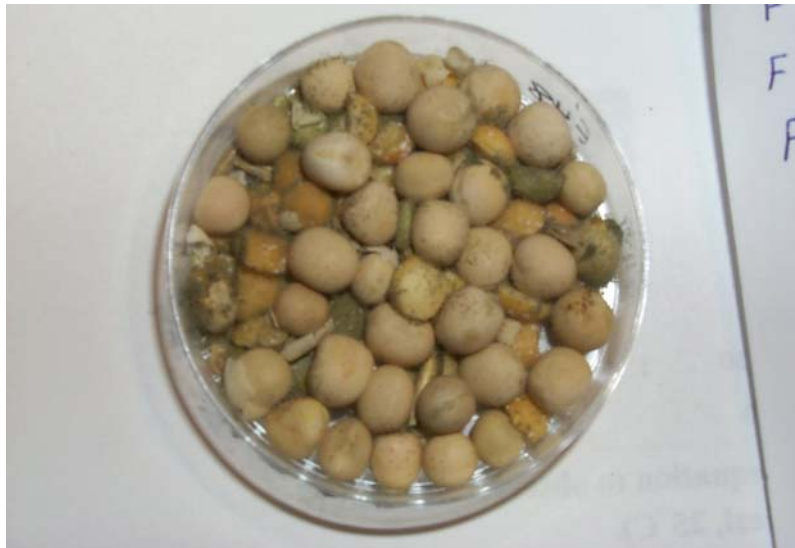
Figure 4.11 Feed-grade pea molded at 40°C and 90% RH.
