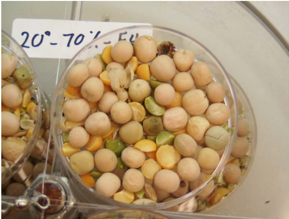
Figure E.5 Appearance of clean and feed peas after 216 days of storage at 20°C and 70% RH.
