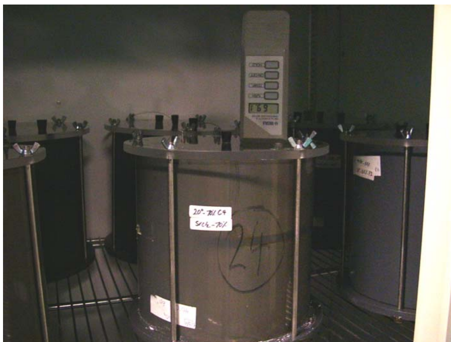
Figure 4.8 Measuring of the RH within the airtight chamber.
