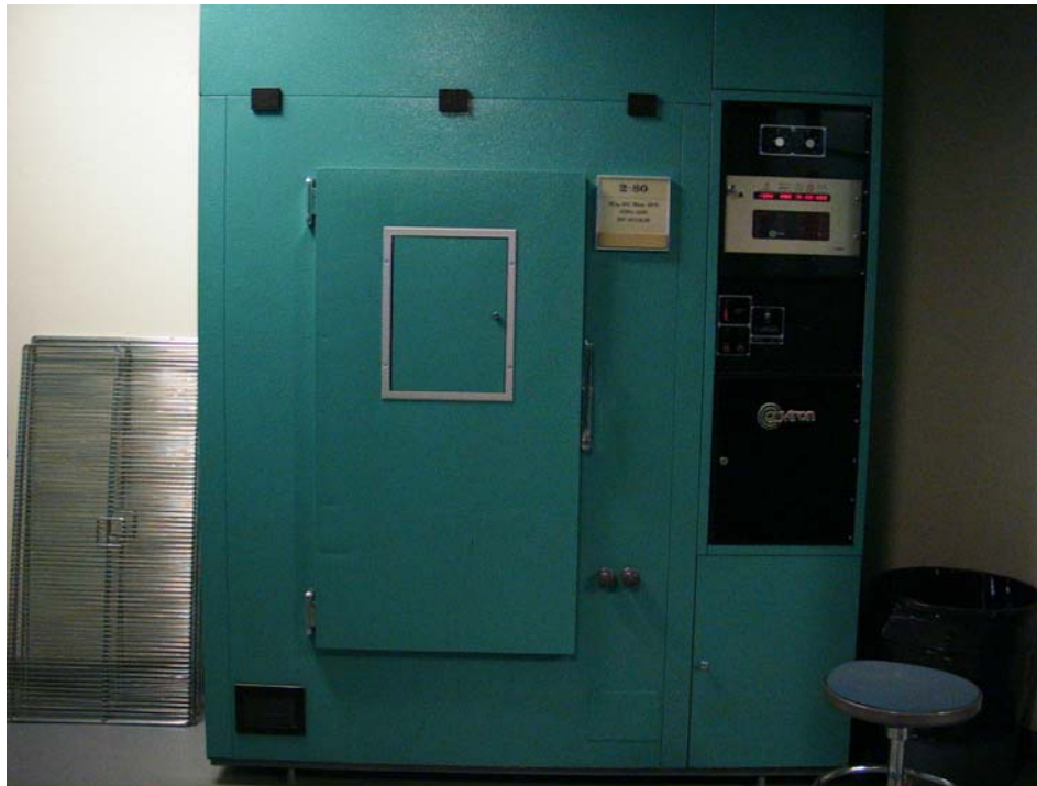
Figure 4.5 Controlled environment chamber.
