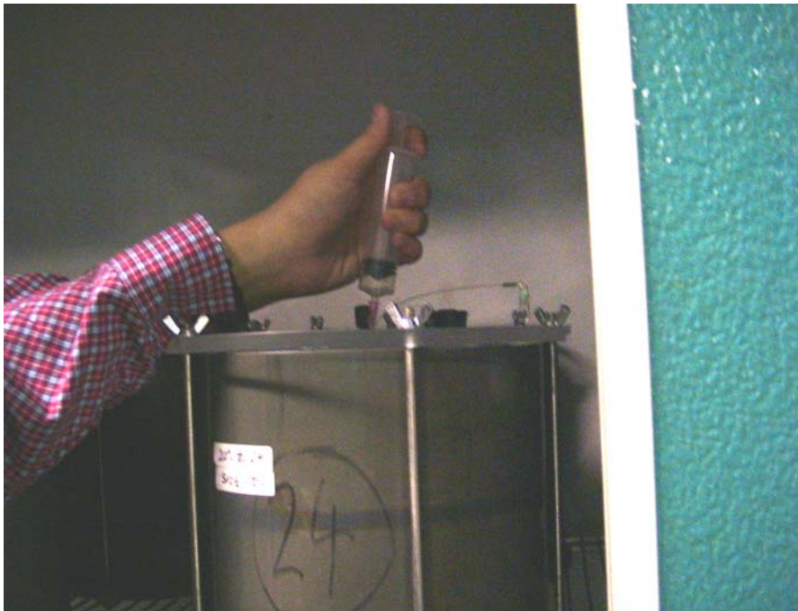
Figure 4.10 Taking CO 2 sample by inserting a 20 mm syringe beside the rubber stopper.
