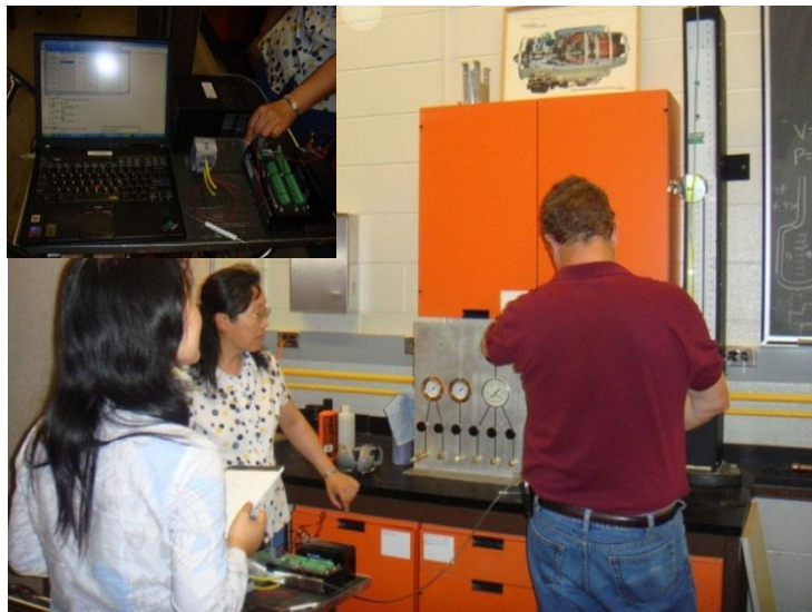
Figure B.2 Calibration of the pressure transducer
