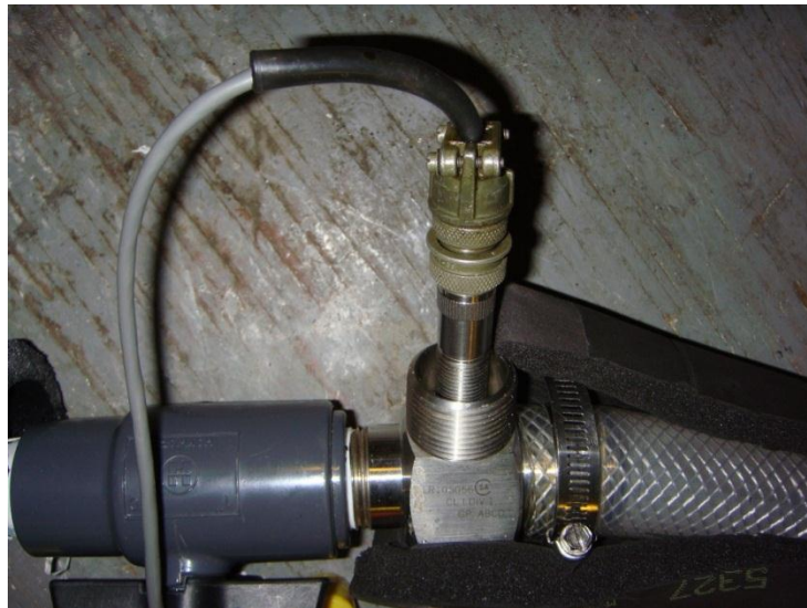
Figure A.2 Hedland model 1100 turbine flow meter
