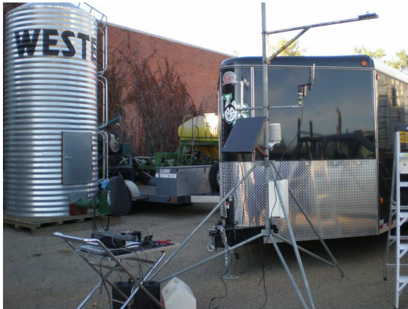
Figure B.1 Calibration of temperature and relative humidity sensors and pyranometers
