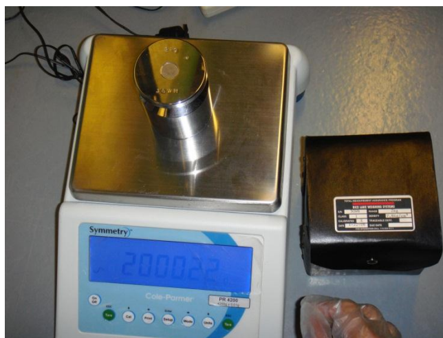
Figure A.4 Calibration of the digital scale
