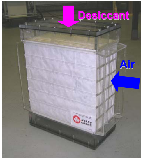
Figure 1-4. RAMEE Prototype 1 (Hemingson, 2005).
