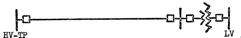
Figure 4.8 Building a Line from a High Voltage Terminal Priority (HV-TP) Bus to the Low Voltage (LV) Bus
