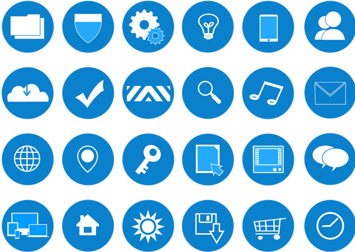
Figure 2.5: Example of flat interface. Visual variables such as colour, contrast, weight, and size are repeated across the entire set. Abstract (triangles dispersing outwards) and concrete (clock for timer) meaning can be observed in the interface. From “Icons Web Development Website Design Flat” [4].
