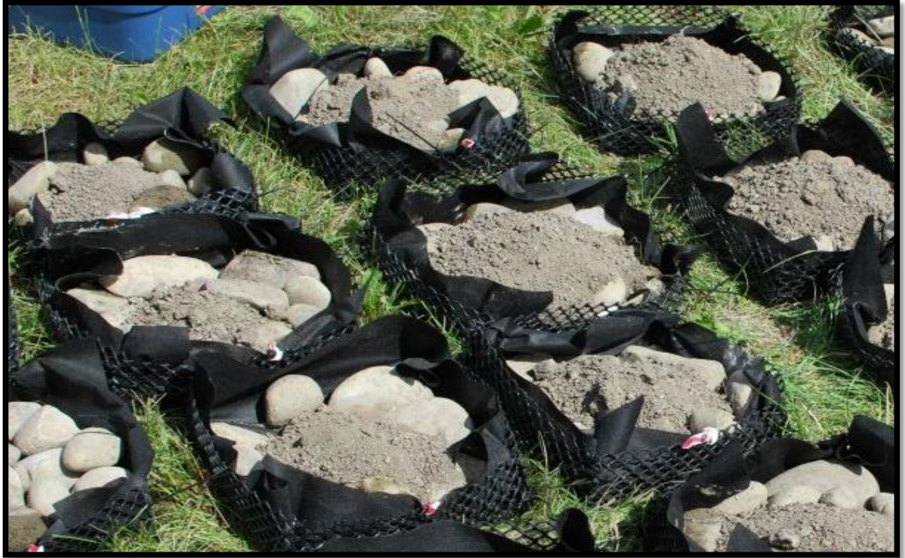
Fig. 2: Cobble baskets deployed June 5, 2012 at Eyebrow Marsh in the Upper Qu'Appelle River. Sediment depths range from control (left) with no sediment added to smothered (right) with 2400 mL sediment added.
