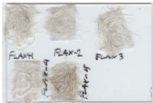
Figure 3.14 Photograph of the samples used for XRD test.
