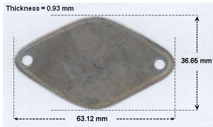
Figure 3.7 Dimensions of the upper electrode.
