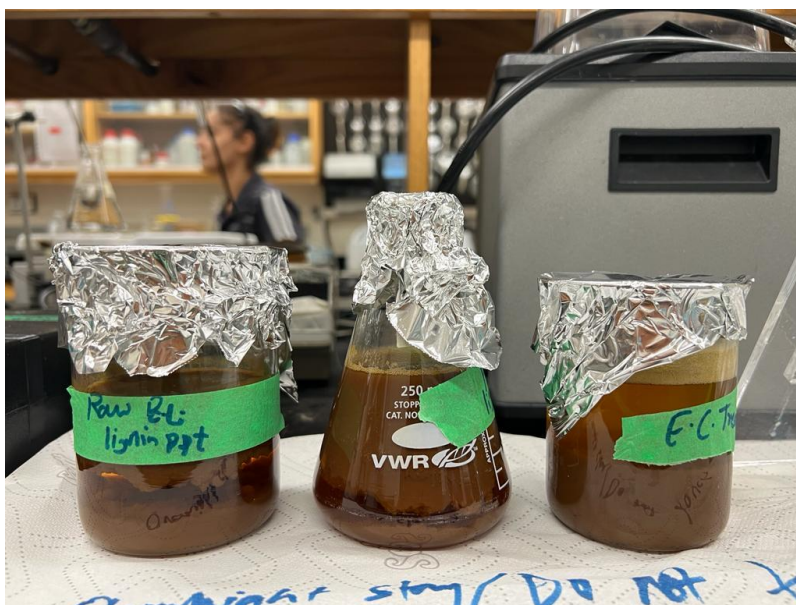
Figure D4 Lignin Precipitation of BL Samples by Acid Hydrolysis
