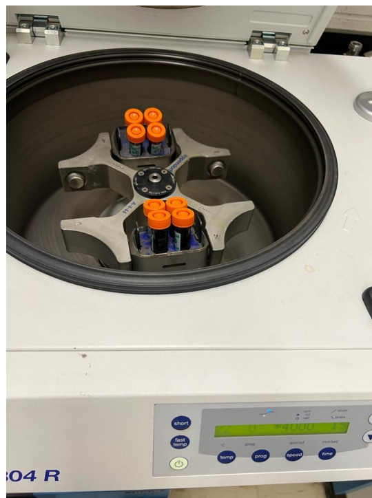
Figure D10 Centrifugation of Anaerobically Digested BL Samples using Centrifuge 5804 R
