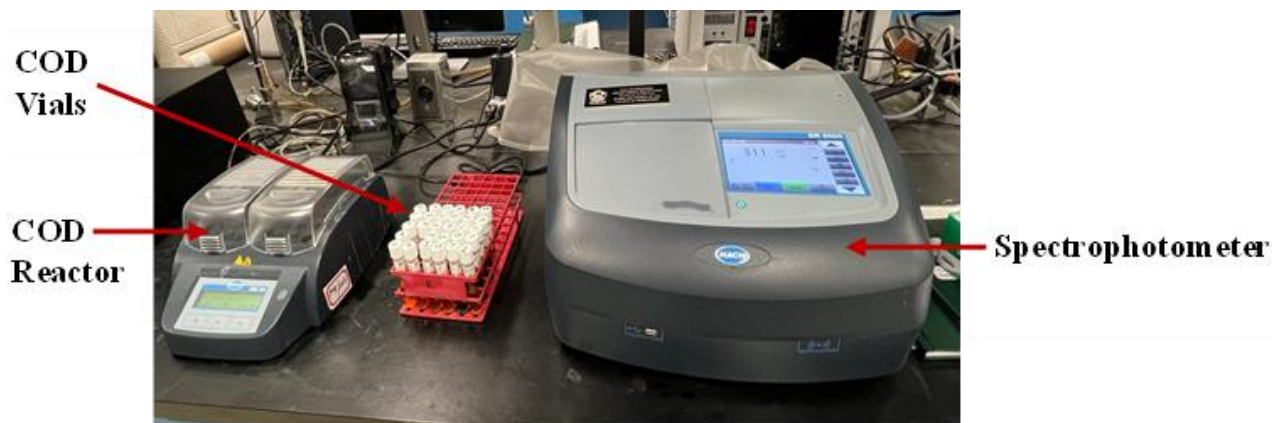
Figure 3.5 Chemical Oxygen Demand (COD) Analyzing Unit
