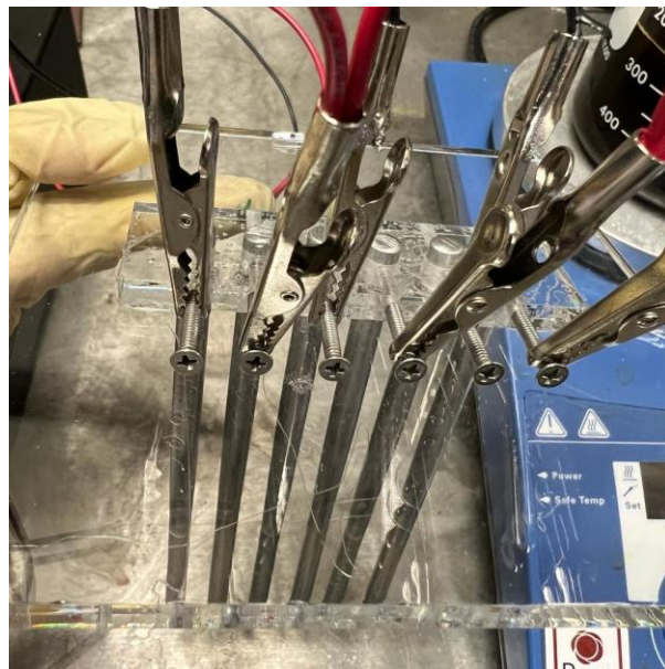
Figure D4 Alternate anode and cathode connection to the Electrodes
