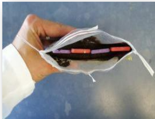
Figure 3. Western Ag Labs Ltd. 24-hour nutrient supply rate measurement using PRS™-probes
