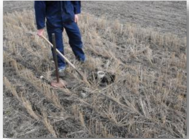
Figure 2. Inserting and extracting a PVC core to collect undisturbed soil for the incubation study
