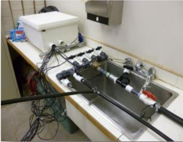
Figure 4. Automated watering system to maintain soils at field capacity
