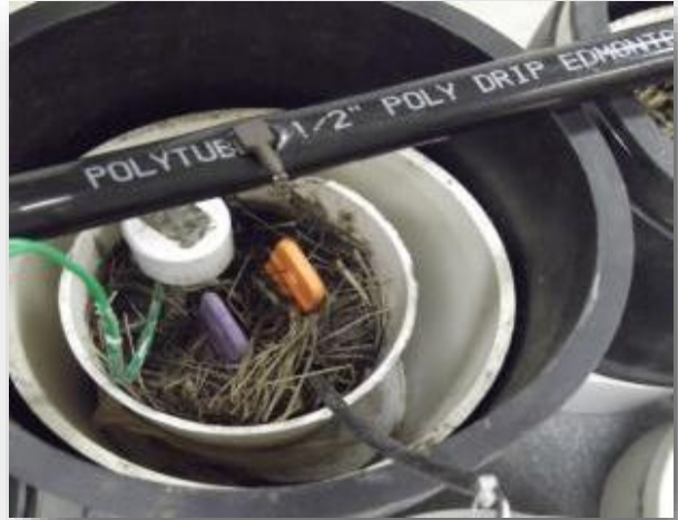
Figure 4. Automated watering system to maintain soils at field capacity
