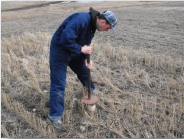
Figure 2. Inserting and extracting a PVC core to collect undisturbed soil for the incubation study
