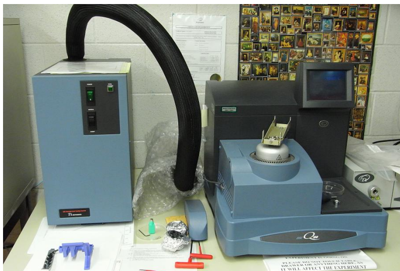
Figure 3.4: A differential scanning calorimeter (Q100, TA Instruments).
