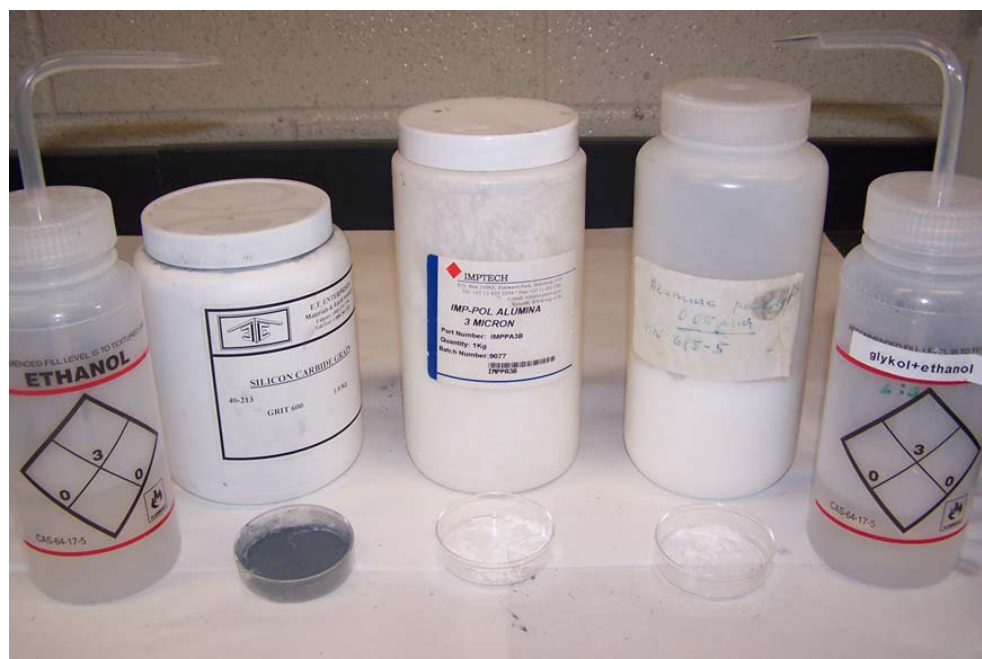
Figure 3.7: Materials used for polishing. From left to right: 100 % ethanol, silicon carbide powder, 3 micron alumina powder, 0.05 micron alumina powder and an ethanol + glycol mixture. The image was extracted from [48].
