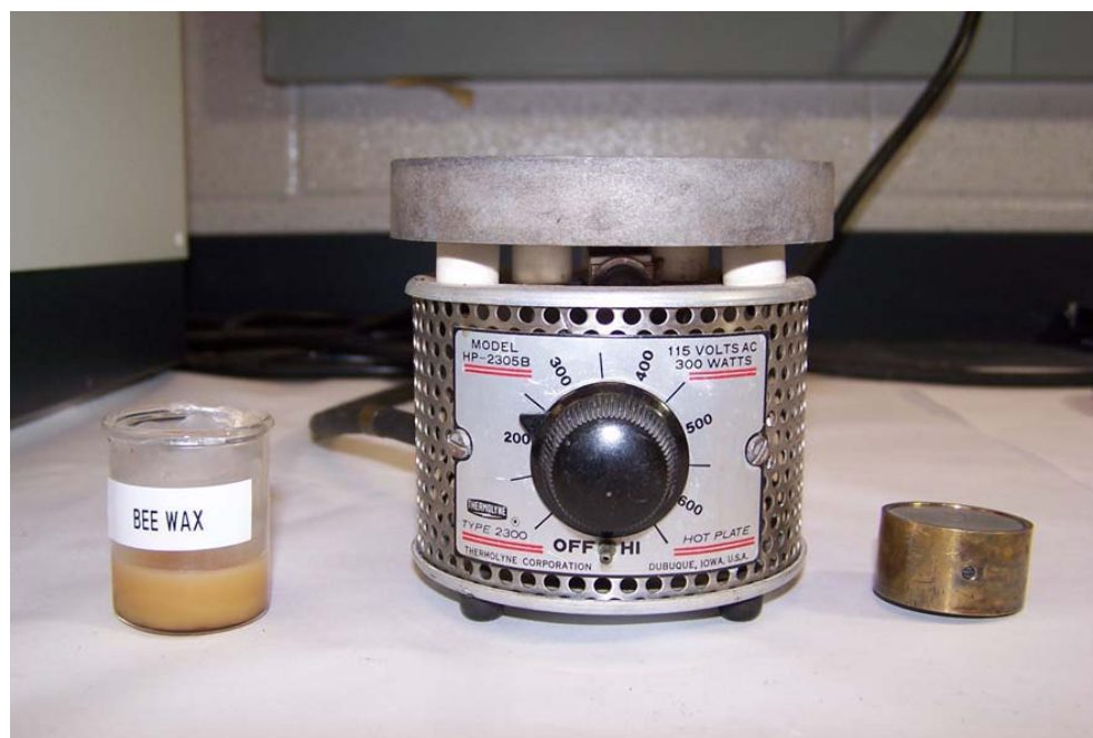
Figure 3.6: From left to right: Bee's wax, a heater (Thermolyne HP2305B), and a sample holder. The image was extracted from [48].
