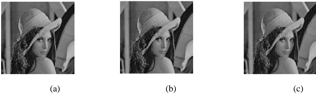
Figure 5.20 (a) original “Lena” image; (b) 8-bit AIQ (PSNR = 89.5 dB); and (c) 8-bit FP (PSNR = 80 dB) implementation
