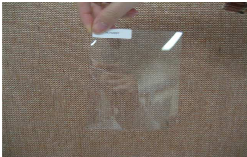
Figure 3-1: Transparent pure SWNT film purchased from Unidym Inc
