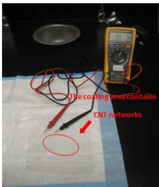
Figure 4-6: Identify the coating area which contains CNT networks by a multimeter
