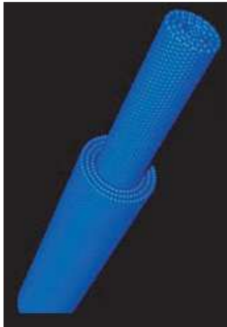
Figure 2-6: Schematic structure of a multiwall carbon nanotube (MWNT) ( http://chattahbox.com/images/2009/06/carbon_nanotubes.jpg )
