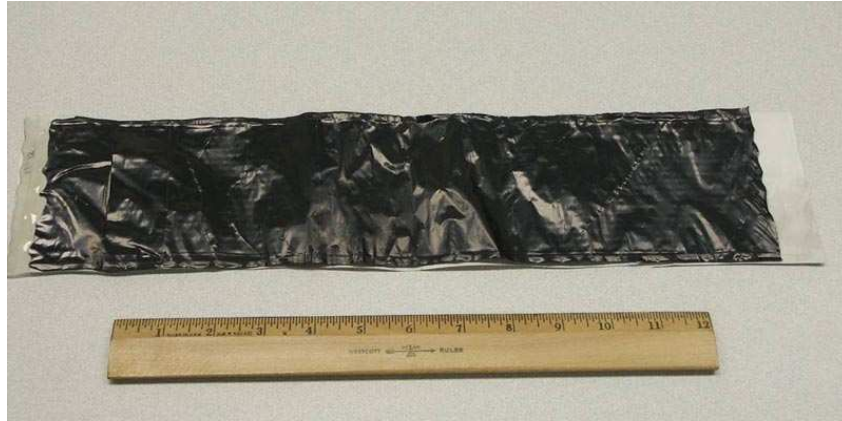
Figure 2-12: A product of “Buckypaper” fabricated by the method proposed by Dharap et al. (2004)
