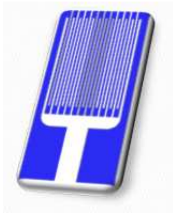
Figure 2-3: A model of a typical metallic strain gauge
