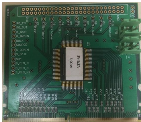
Figure 5.1 Photo of PCB with the SRAM chip soldered
