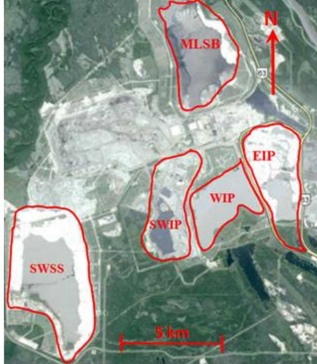
Figure 1.2: Tailings and process water areas at Mildred Lake Mine (Google 2013a) Abbreviations: EIP= East in-Pit, WIP= West in-pit, SWIP= Southwest in-pit, SWSS= Southwest Sands Storage, MLSB= Mildred Lake Settling Basin
