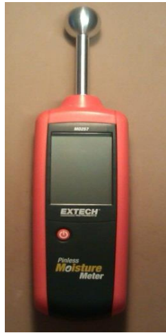
Figure 3.5 The Exetch MO257 moisture sensor with the ball shaped sensor at the top of the device
