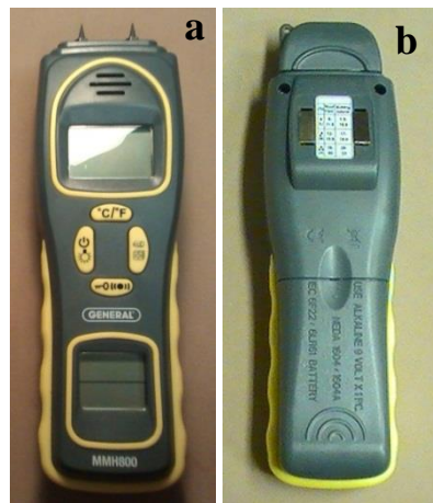
Figure 3.4 The general MMH800 sensor. Pin sensors are located at the top (a) and a pad sensor is located at the back (b) of the device.
