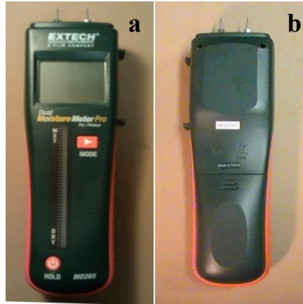
Figure 3.6 The Extech MO265 sensor. Pin sensors are located at the top (a) and a pad sensors is located at the back of the device (b)
