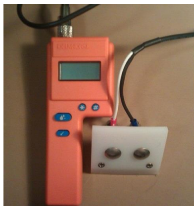
Figure 3.3 Delmhorst FX-2000 Hay moisture meter. The sensors are located on the white pad.
