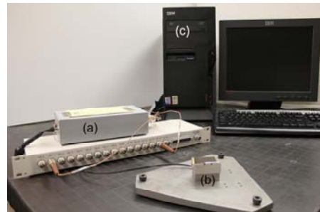
Fig. 2. Experiment setup including (a) a power amplifier E-625.CR, (b) the P-753 PEA, and (c) a computer with the PCI-DAS1602/16 I/O board.
