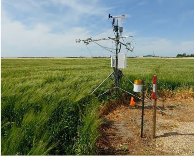
Figure 21. Eddy-covariance meteorological station at the barley field
