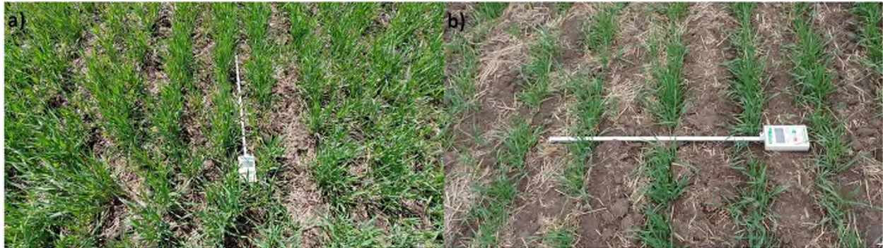
Figure 8. Example of field LAI measurements a) with-row and b) cross-row
