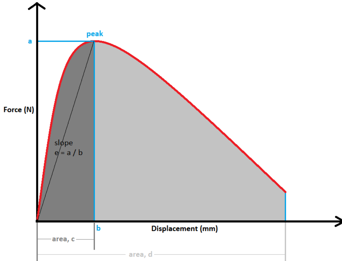
Figure 4.2 Example load-displacement curve of three-point bending test.
