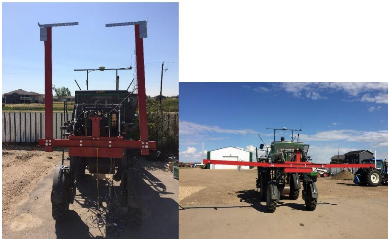
Figure 1-4: 2nd Generation Boom. Left: Folded Form, Right: Open Form. Picture Credit: Robotics Lab, U of S
