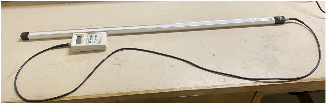
Figure 4.3: LI-COR line quantum sensor and LI-COR LI-250 light meter
