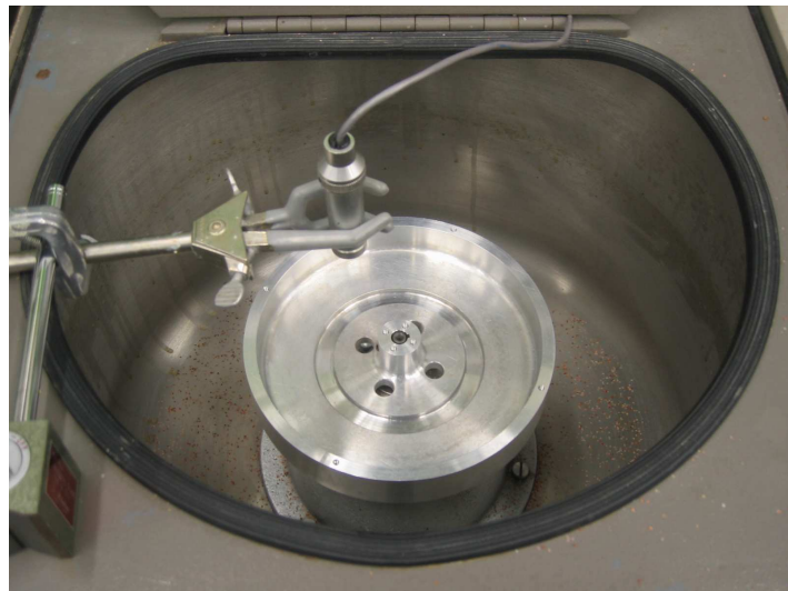
Figure 2-11: Experimental apparatus to measure fracture rotating speed including the centrifuge, aluminium holder and non-contact tachometer
