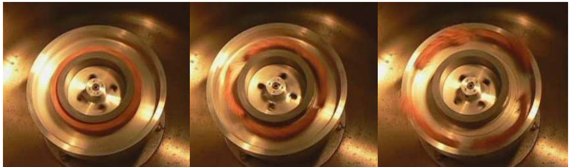
Figure 2-13: A sequence of three photos (30 frames per second) which captured the potash caked ring just before and after the instant fracture in the centrifuge, \omega \approx 250rpm
