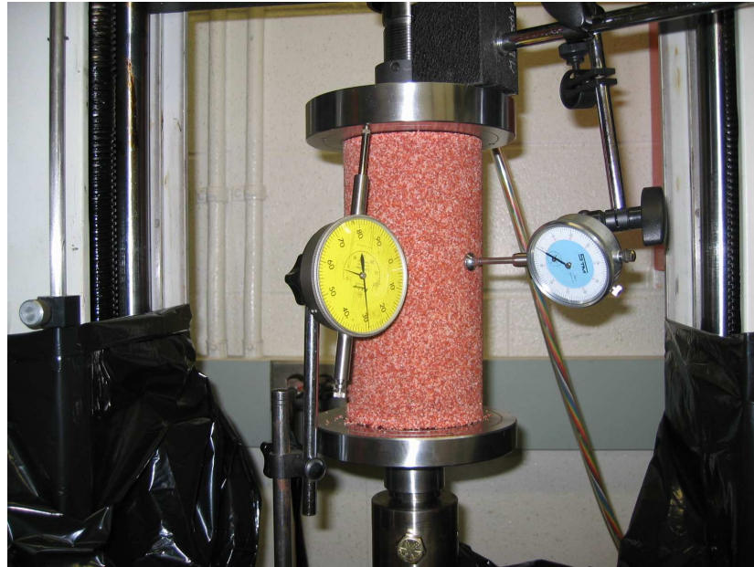
Figure B-1: Compression test in the INSTRON machine used to determine Young's modulus and Poisson's ratio for a caked potash sample
