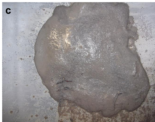
Figure 3. Heavy clay soil cores prior to manual washing without pre-treatment (a) or shaken in solution for 15 min with either deionized water (b) or 1.2M NaHCO 3 (c).
