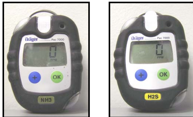
Figure C.5 Ammonia (NH 3 ) and hydrogen sulfide (H 2 S) monitors
