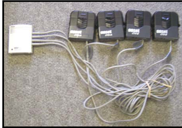
Figure C.2 Split-core current transducers (CTs) and datalogger
